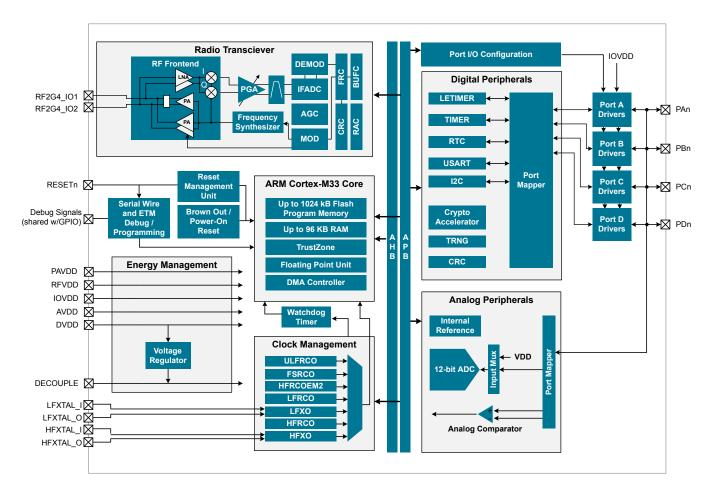
Figure 3.1. Detailed EFR32MG21 Block Diagram
