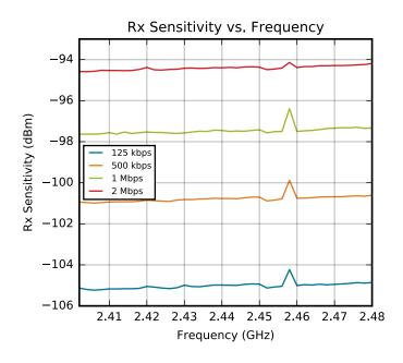
Figure 4.10. 2.4 GHz BLE RF Receiver Sensitivity
