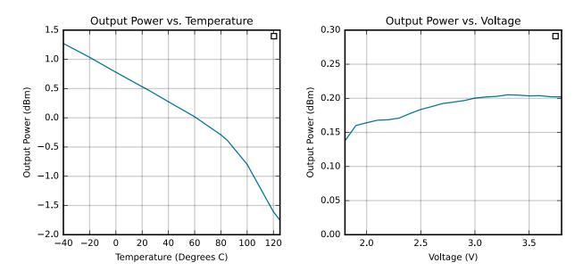
Figure 4.18. 2.4 GHz 0 dBm PA RF Transmitter Output Power
