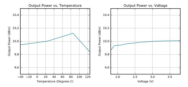
Figure 4.7. 2.4 GHz 10 dBm PA RF Transmitter Output Power
