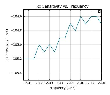
Figure 4.19. 2.4 GHz 802.15.4 RF Receiver Sensitivity
