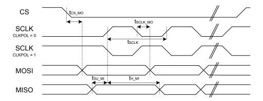
Figure 4.11. SPI Main Timing (SMSDELAY = 0)
