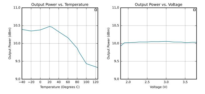
Figure 4.17. 2.4 GHz 10 dBm PA RF Transmitter Output Power
