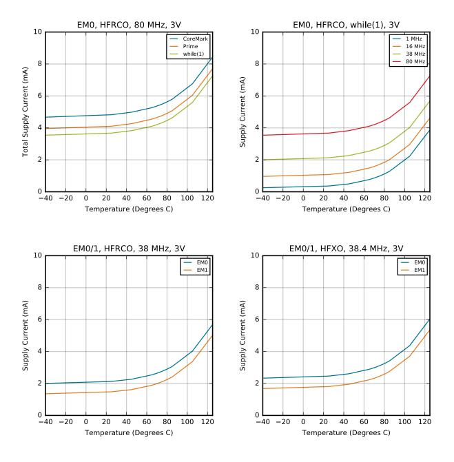
Figure 4.14. EM0 Active Mode Typical Supply Current vs. Temperature
