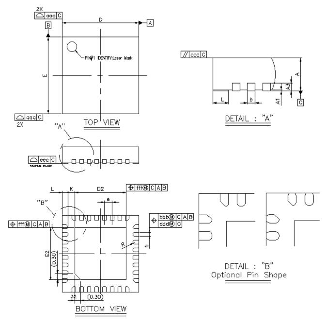
Figure 7.1. QFN32 Package Drawing
