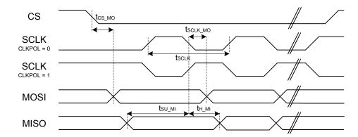
Figure 4.12. SPI Main Timing (SMSDELAY = 1)
