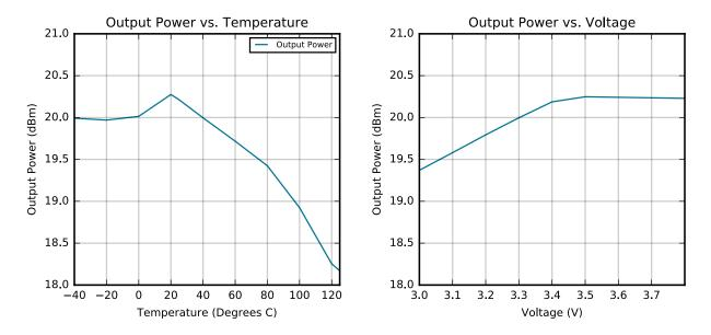
Figure 4.16. 2.4 GHz 20 dBm PA RF Transmitter Output Power
