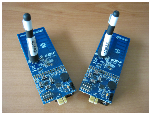
Figure 27. 4455-LED-434 Pico Boards used for the Range Tests
