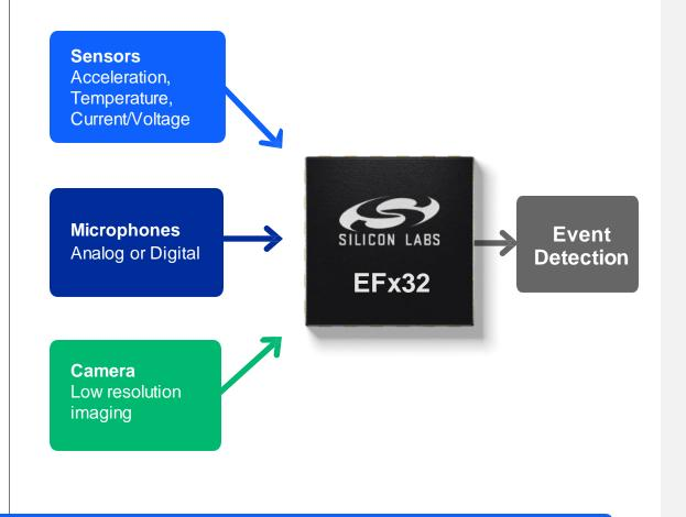
AI/ML Hardware Accelerator enables efficient Edge ML inferencing
