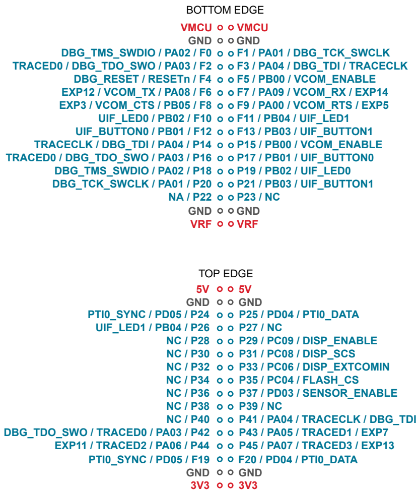
Figure 3.3. Wireless Pro Kit Mainboard (BRD4002A) Breakout Pad Pin Mapping
