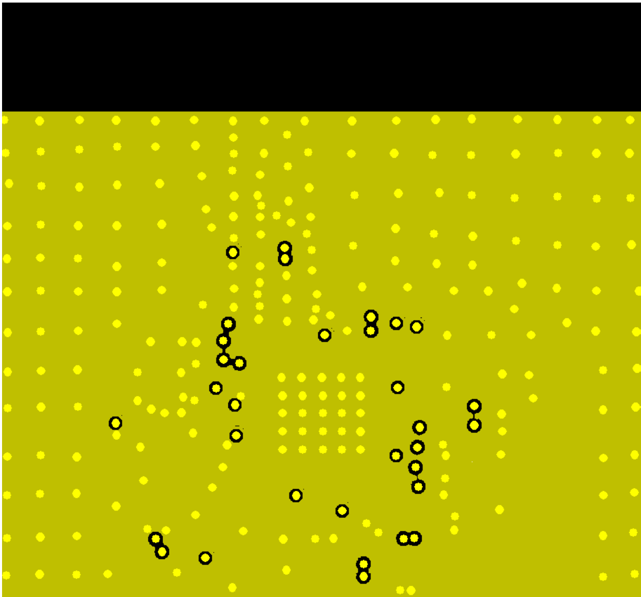
Figure 11: GND Plane in Layer 2
