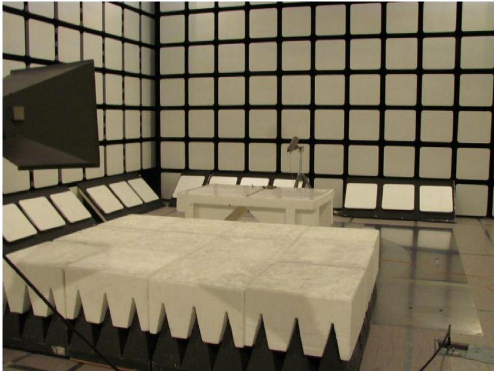
Photograph 3. Radiated immunity test set-up (1.4 to 2.7 GHz).
