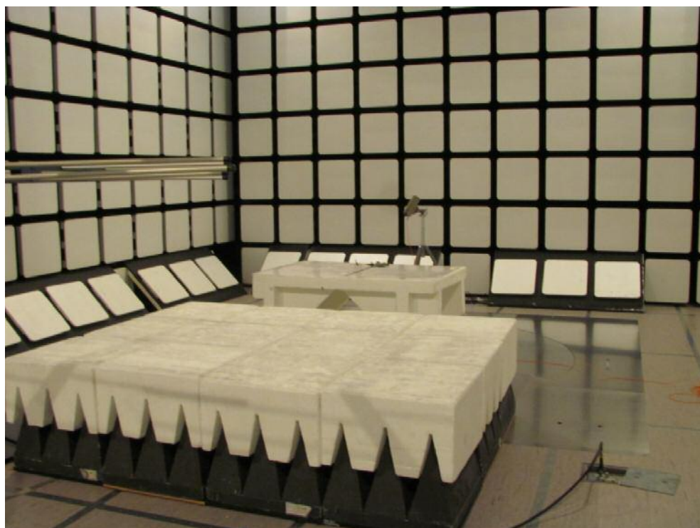
Photograph 2. Radiated immunity test set-up (80 to 1000 MHz).
