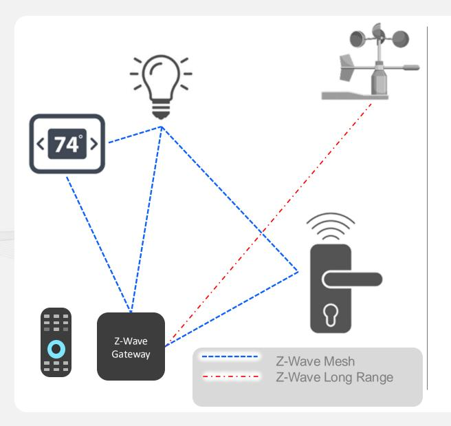
New Long-Range channel in Z-Wave DSSS-OQPSK PHY; 100 kbps data rate Up to +30 dBm TX power [FCC 15.247]
