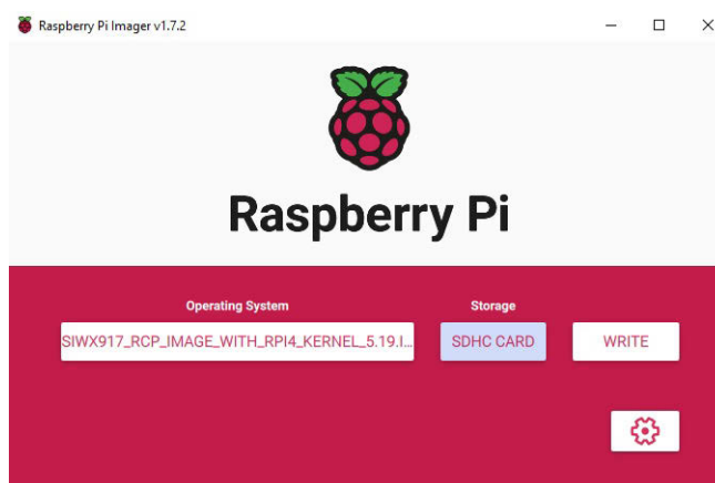
Figure 4.4. Write to SD card
