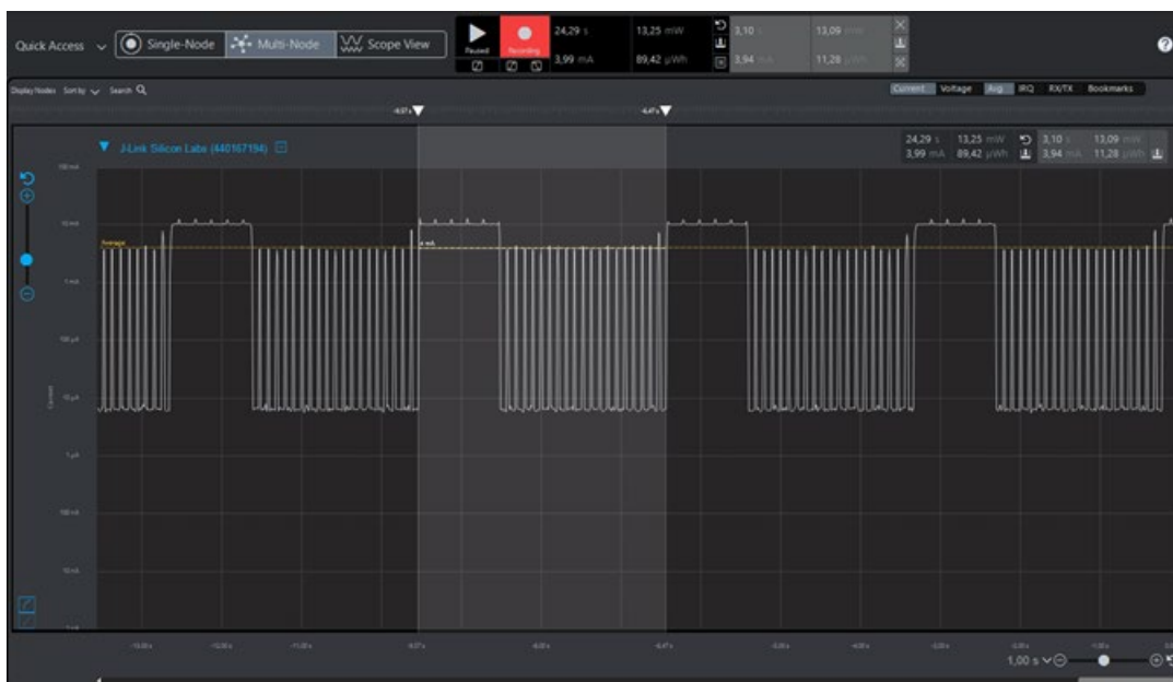
Figure 3.2. Current Profile for EFR32xG21 Series 2, Looking for a Friend Node, with Proxy
