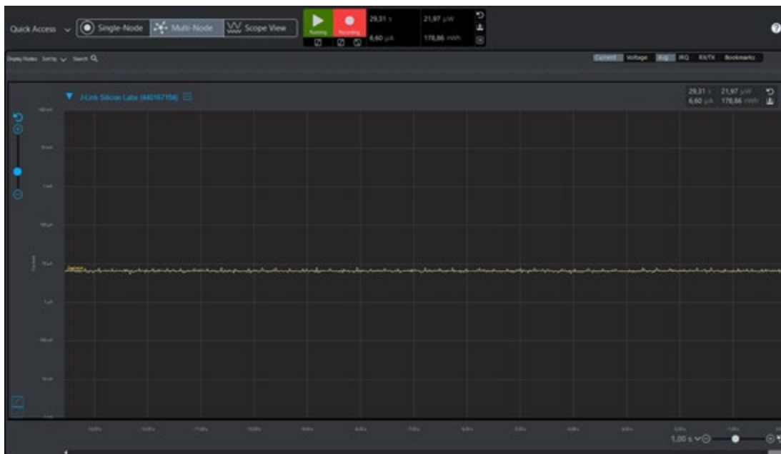
Figure 3.4. Current Profile for EFR32xG21 Series 2, Friendship established, no Proxy
