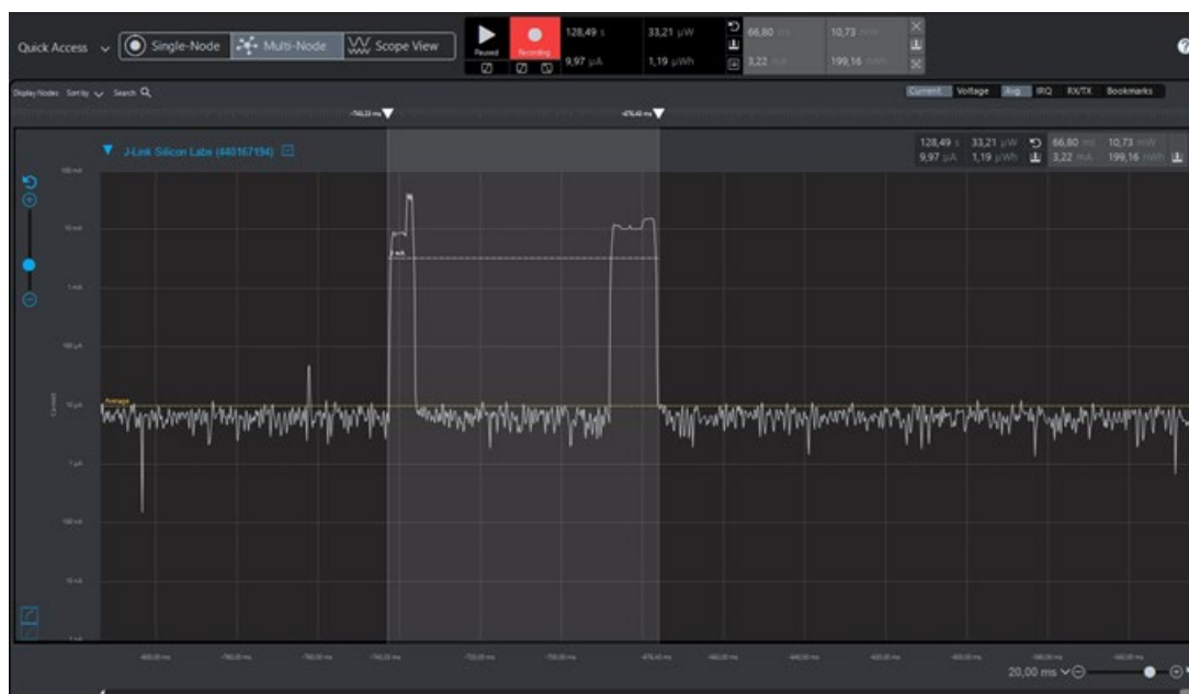
Figure 3.6. Current Profile for EFR32xG21 Series 2, Friendship established, no Proxy, Friend Poll & Update
