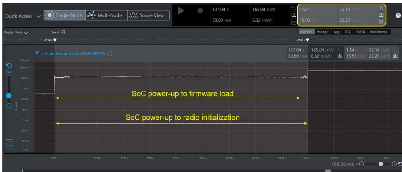
Figure 7.2. SiWG917 Current Consumption during Initialization
