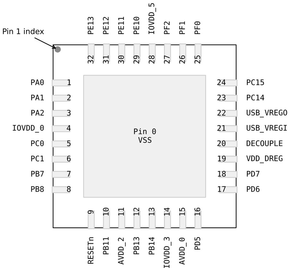
Figure 5.7. EFM32HG310 Pinout (top view, not to scale)
