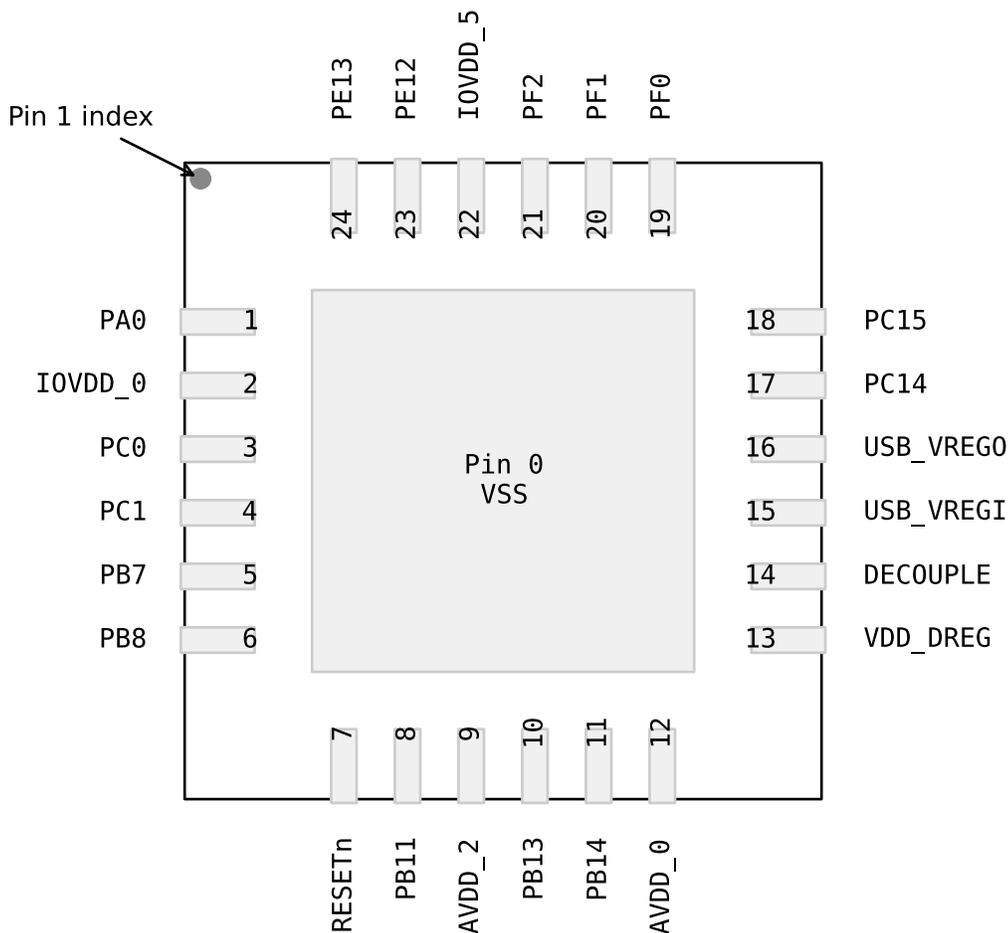
Figure 5.5. EFM32HG308 Pinout (top view, not to scale)
