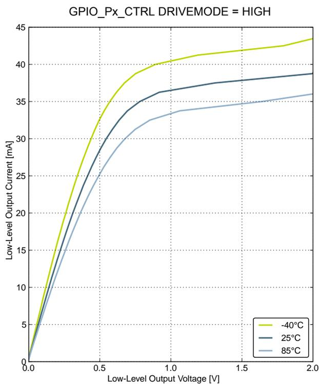
Figure 4.14. Typical Low-Level Output Current, 2V Supply Voltage
