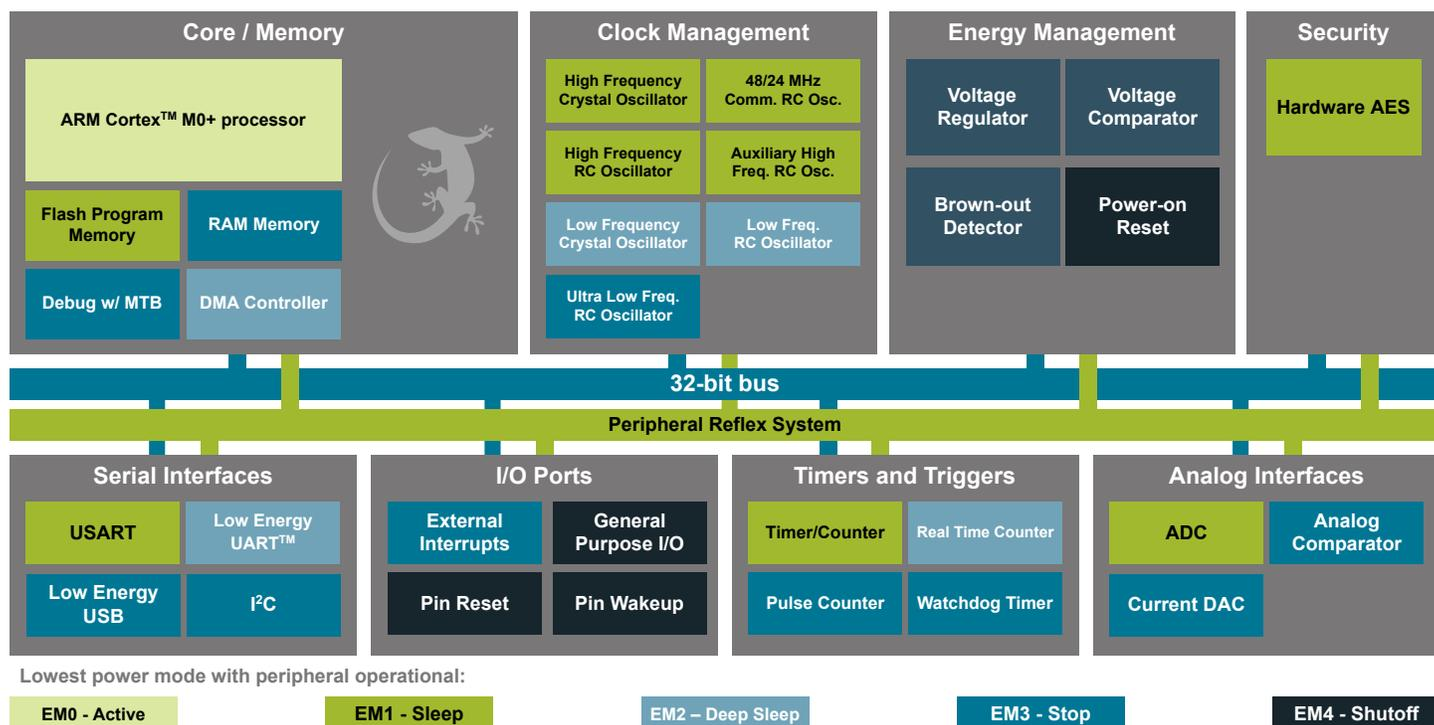
Figure 3.1. Block Diagram
