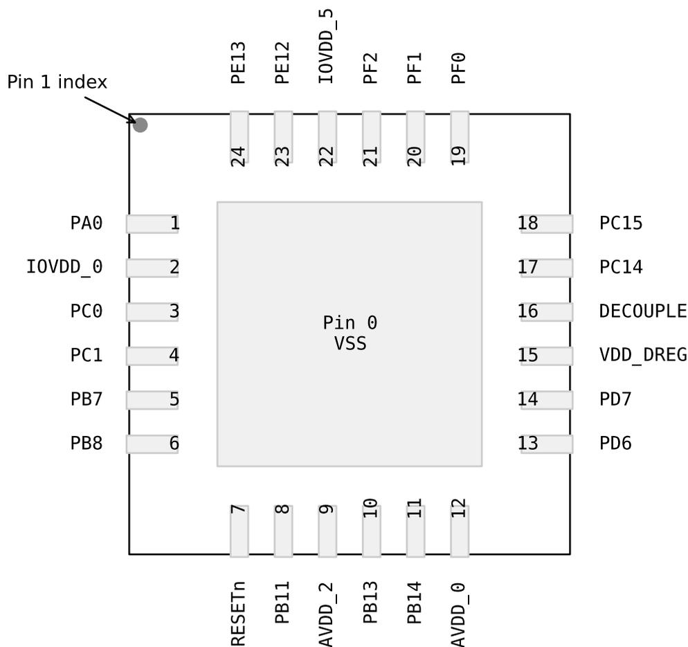
Figure 5.2. EFM32HG110 Pinout (top view, not to scale)
