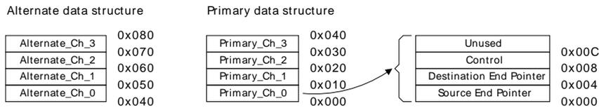
This structure in Figure 8.6 (p. 58) uses bytes of system memory. The controller uses the lower 8 address bits to enable it to access all of the elements in the structure and therefore the base address must be at 0xXXXXXX00.
