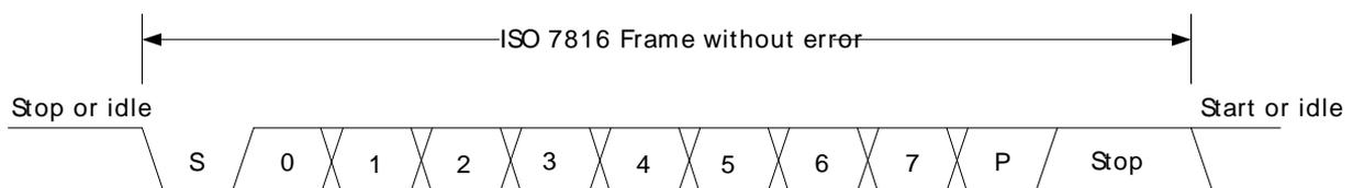
If a parity error is detected by the receiver, it pulls the line I/O line low after half a stop bit, see Figure 16.13 (p. 342). It holds the line low for one bit-period before it releases the line. In this case, the guard time is extended by one bit period before a new transmission can start, resulting in a total of 3 stop bits.
