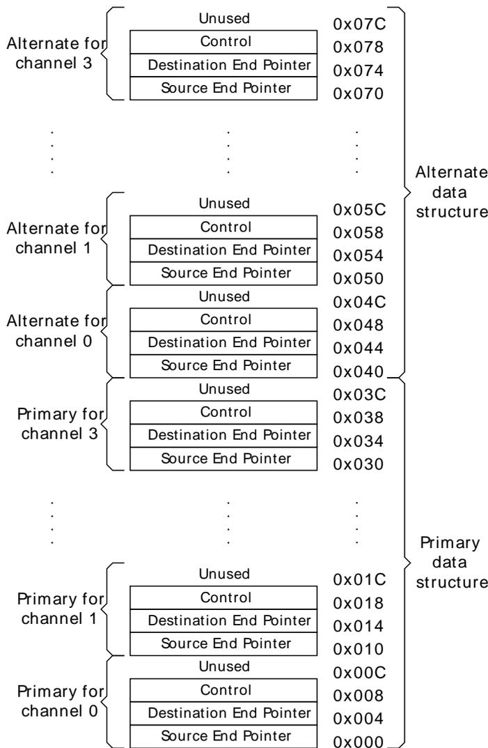
The controller uses the system memory to enable it to access two pointers and the control information that it requires for each channel. The following subsections will describe these 32-bit memory locations and how the controller calculates the DMA transfer address.
