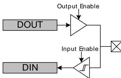
When MODEn is 0110 or 0111, the pin operates in open-source mode, the latter with a pull-down resistor. When driving a high value in open-source mode, the pull-down is disconnected to save power.
