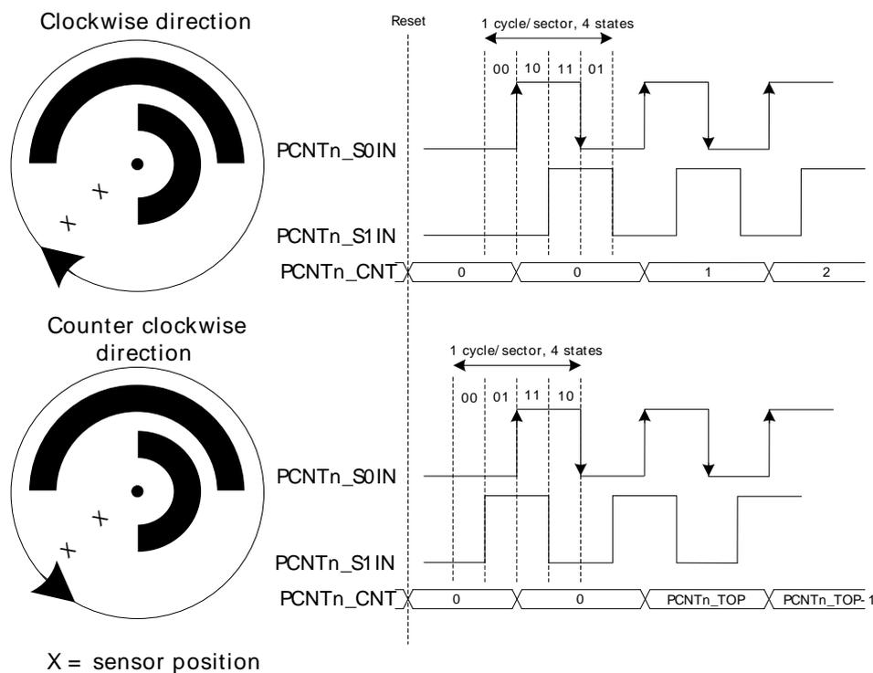
If PCNTn\_S0IN leads PCNTn\_S1IN in phase, the direction is clockwise, and if it lags in phase the direction is counter-clockwise. Although the direction is automatically detected, the detected direction may be inverted by writing 1 to the EDGE bit in the PCNTn\_CTRL register. Default behavior is illustrated by Figure 20.2 (p. 448) .
