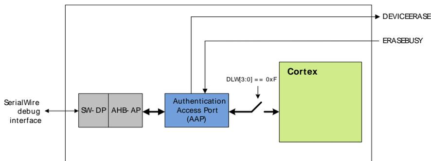
As seen from Figure 6.1 (p. 24), the AAP is situated after the AHB-AP, meaning it should be accessed like any other peripheral from the debug. The address of the AAP is 0xF0E00000 as can also be seen from Figure 5.2 (p. 16).
