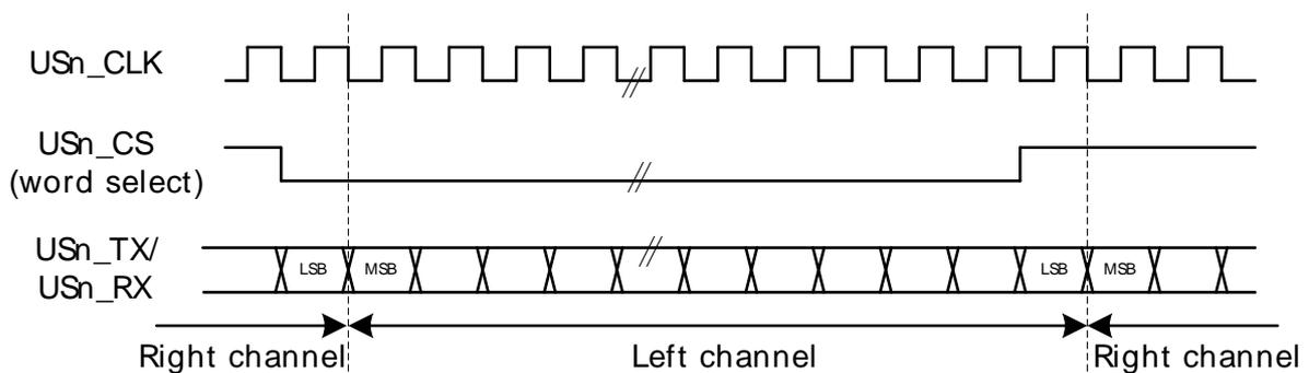
**Figure 16.19. USART Standard I2S waveform (reduced accuracy)**
