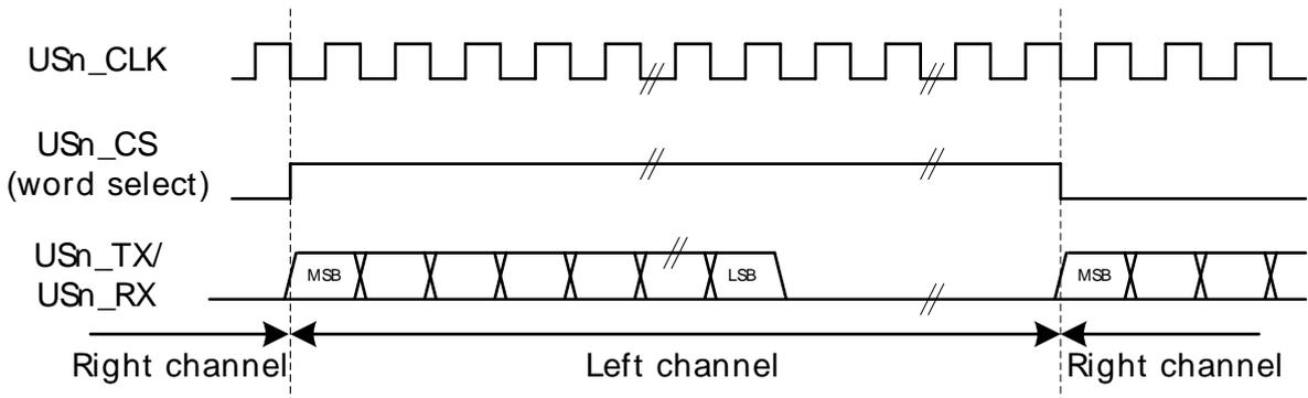
A right-justified stream is shown in Figure 16.21 (p. 348) . The left and right justified streams are equal when the data-size is equal to the word-width.
