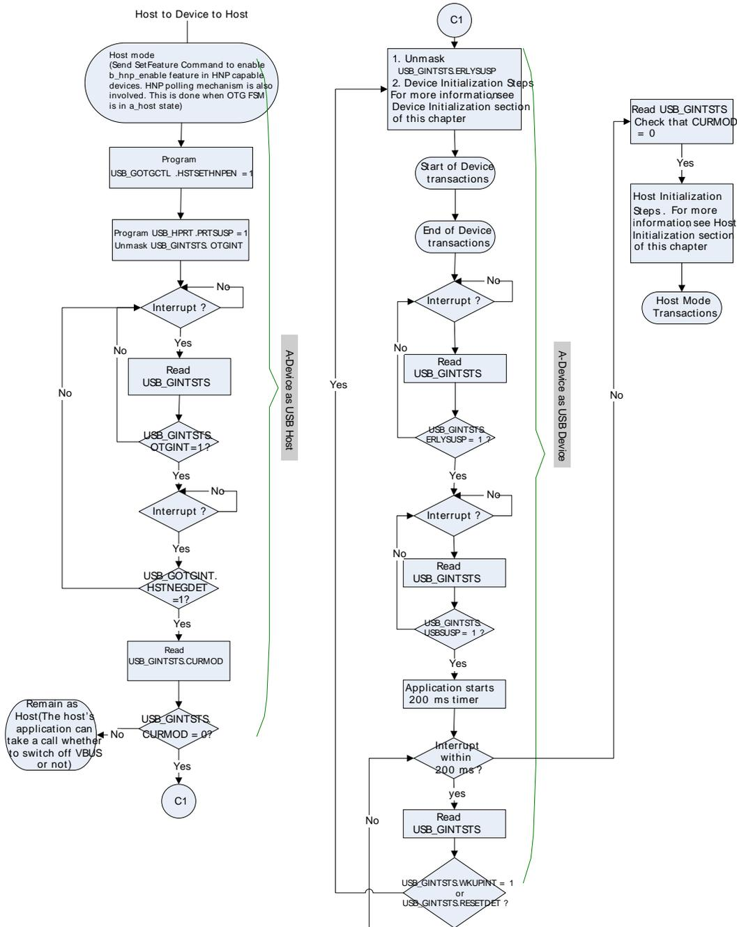
Figure 14.32 (p. 231) shows the programming steps that need to be performed by B-device's application (core as B-device) in order to change its role to Host. In Figure 14.32 (p. 231) , the B-device performs a role change, becomes a Host and then reverts back to Device mode of operation.
