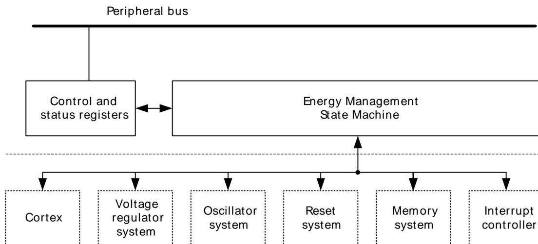
The EMU is available as a peripheral on the peripheral bus. The energy management state machine is triggered from the Cortex-M0+ and controls the internal voltage regulators, oscillators, memories and interrupt systems in the low energy modes. Events from the interrupt or reset systems can in turn cause the energy management state machine to return to its active state. This is further described in the following sections.
