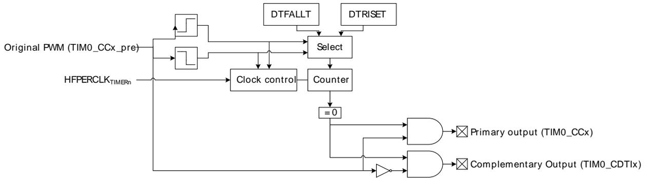
The DTI unit is enabled by setting DTEN in TIMER0\_DTCTRL. In addition to providing the complementary outputs, the DTI unit then also overrides the compare match outputs from the timer.
