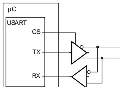
The USn\_CS output is active low by default, but its polarity can be changed with CSINV in USARTn\_CTRL. AUTOCS works regardless of which mode the USART is in, so this functionality can also be used for automatic chip/slave select when in synchronous mode (e.g. SPI).
