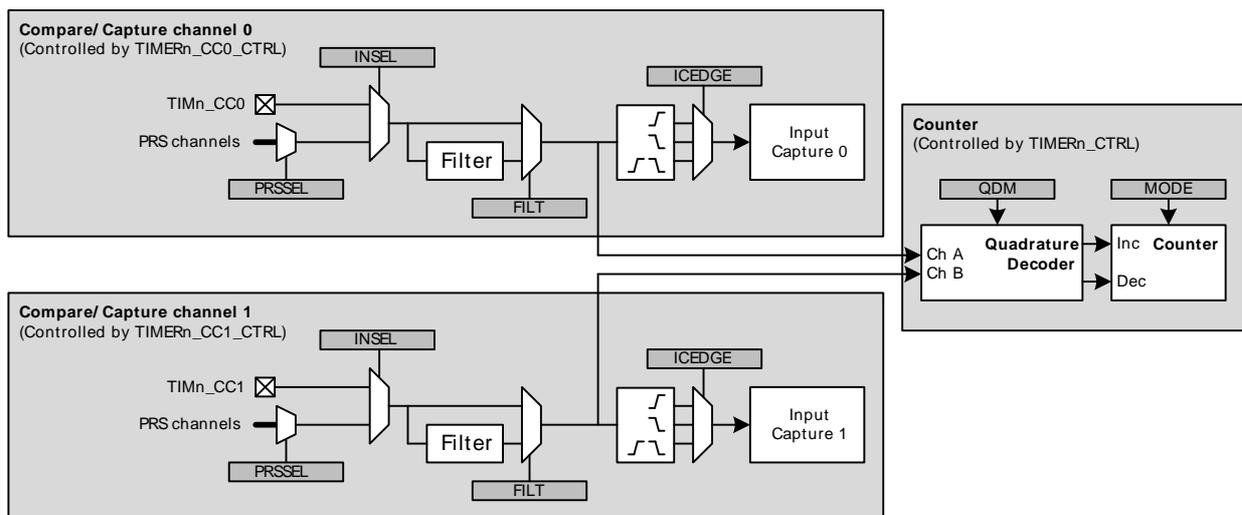
The Quadrature Decoder can be set in either X2 or X4 mode, which is configured in the QDM bit in TIMERN\_CTRL. See Figure 18.7 (p. 404)
