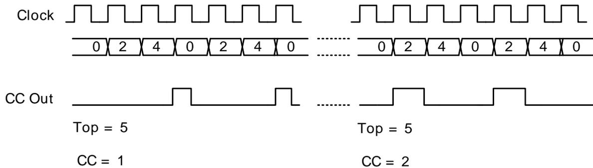
The mode is enabled by setting the X2CNT field in TIMERN\_CTRL register. The intended use of the 2x mode is to generate 2x PWM frequency when the Compare/Capture channel is put in PWM mode. Since the PWM output is updated on both edges of the clock, frequency prescaling will result in incorrect result in this mode. The PWM resolution (in bits) is then given by Equation 18.6 (p. 411) .
