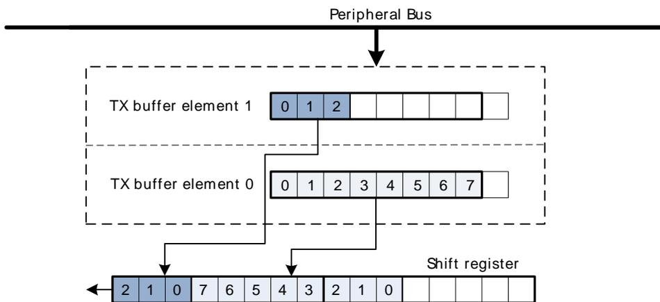
Figure 16.10 (p. 339) illustrates the order of the transmitted bits when an 11 bit frame is transmitted with MSBF set. If MSBF is set and the frame is smaller than 10 bits, only the contents of transmit buffer 0 will be transmitted.
