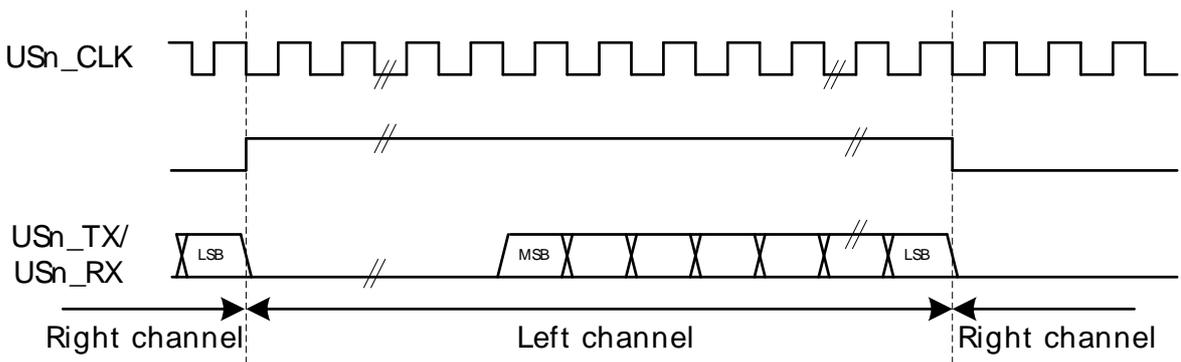
In mono-mode, the word-select signal pulses at the beginning of each word instead of toggling for each word. Mono I2S waveform is shown in Figure 16.22 (p. 349).
