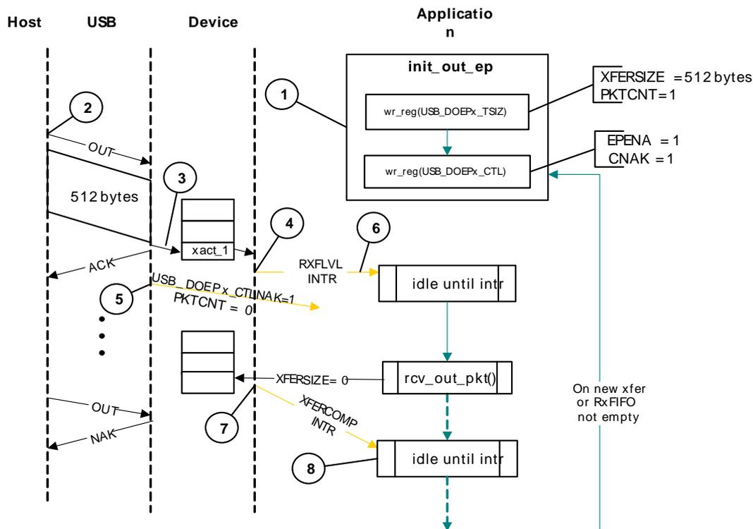
After a SetConfiguration/SetInterface command, the application initializes all OUT endpoints by setting USB\_DOEPx\_CTL.CNAK = 1 and USB\_DOEPx\_CTL.EPENA = 1, and setting a suitable XFERSIZE and PKTCNT in the USB\_DOEPx\_TSIZ register.
