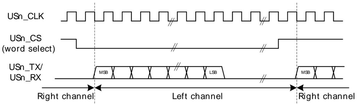
A left-justified stream is shown in Figure 16.20 (p. 348) . Note that the MSB comes directly after the edge on the word-select signal in contradiction to the regular I2S waveform where it comes one bit-period after.
