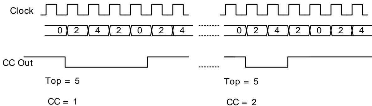
The mode is enabled by setting the X2CNT field in TIMERn\_CTRL register. The intended use of the 2x mode is to generate 2x PWM frequency when the Compare/Capture channel is put in PWM mode. Since the PWM output is updated on both edges of the clock, frequency prescaling will result in incorrect result in this mode. The PWM resolution (in bits) is then given by Equation 18.12 (p. 412) .
