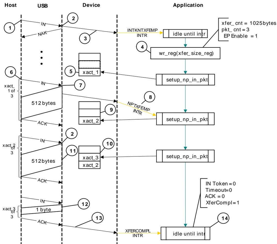
**Slave Mode Bulk IN Two-Endpoint Transfer**
