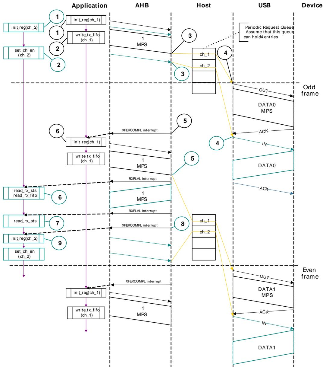
Interrupt Service Routine for Interrupt OUT Transactions in Slave Mode
