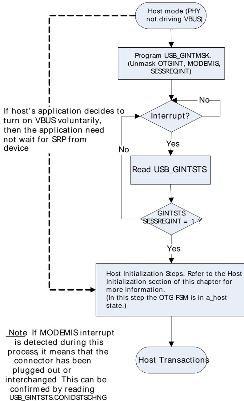
Figure 14.30 (p. 229) illustrates the steps that need to be performed by B-device's application (core as B-device) in order to establishing a connection with A-device by signaling a SRP.
