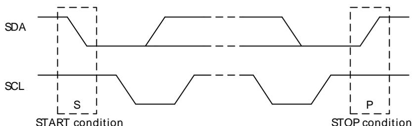
The START and STOP conditions are easily identifiable bus events as they are the only conditions on the bus where a transition is allowed on SDA while SCL is high. During the actual data transmission, SDA is only allowed to change while SCL is low, and must be stable while SCL is high. One bit is transferred per clock pulse on the I<sup>2</sup>C-bus as shown in Figure 15.2 (p. 293).
