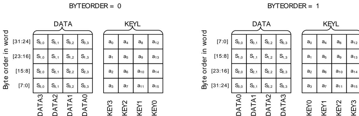
The registers DATA3-DATA0, are not memory mapped directly, but can be written/read by accessing AES\_DATA or AES\_XORDATA. The same applies for the key registers, KEY3-KEY0 which are accessed through AES\_KEYLn (n=A, B, C or D). Writing DATA3-DATA0 is then done through 4
