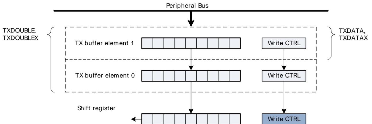
When writing more frames to the transmit buffer than there is free space for, the TXOF interrupt flag in USARTn\_IF will be set, indicating the overflow. The data already in the transmit buffer is preserved in this case, and no data is written.
