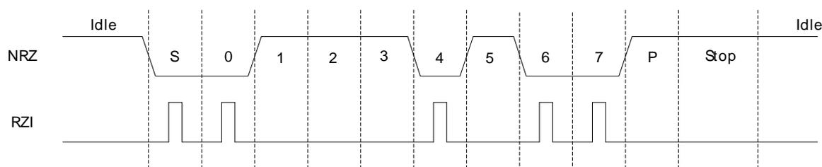
If PULSEEN in LEUARTn\_PULSECTRL is set while INV in LEUARTn\_CTRL is cleared, the output waveform will like RZI shown in Figure 17.7 (p. 384) , only inverted.
