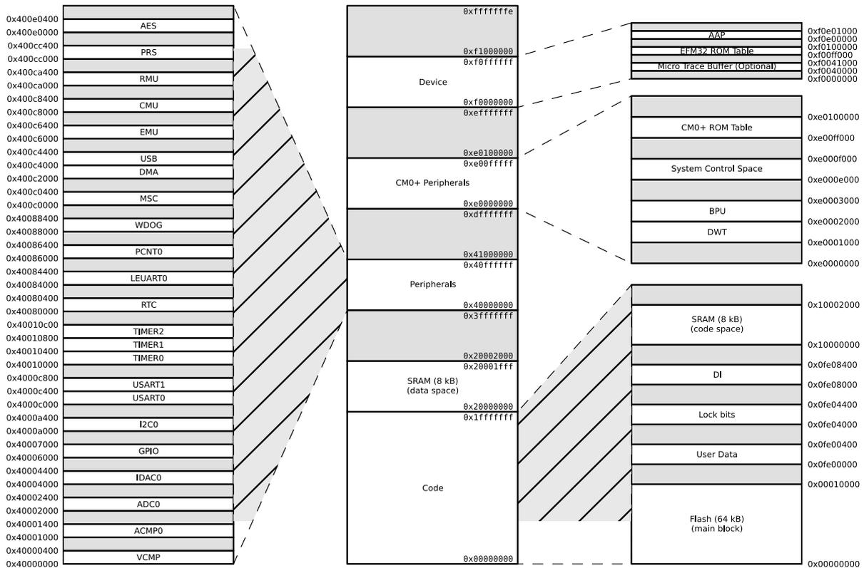
The embedded SRAM is located at address 0x20000000 in the memory map of the EFM32HG. It is also mapped in code space at address 0x10000000 to keep compatibility towards Cortex-M3 and Cortex-M4 EFM32-devices, that uses this code-space mapped SRAM for faster instruction fetching.
