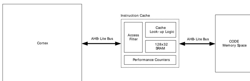
By default, the instruction cache is automatically invalidated when the contents of the flash is changed (i.e. written or erased). In many cases, however, the application only makes changes to data in the flash, not code. In this case, the automatic invalidate feature can be disabled by setting AIDIS in MSC\_READCTRL. The cache can (independent of the AIDIS setting) be manually invalidated by writing 1 to INVCACHE in MSC\_CMD.
