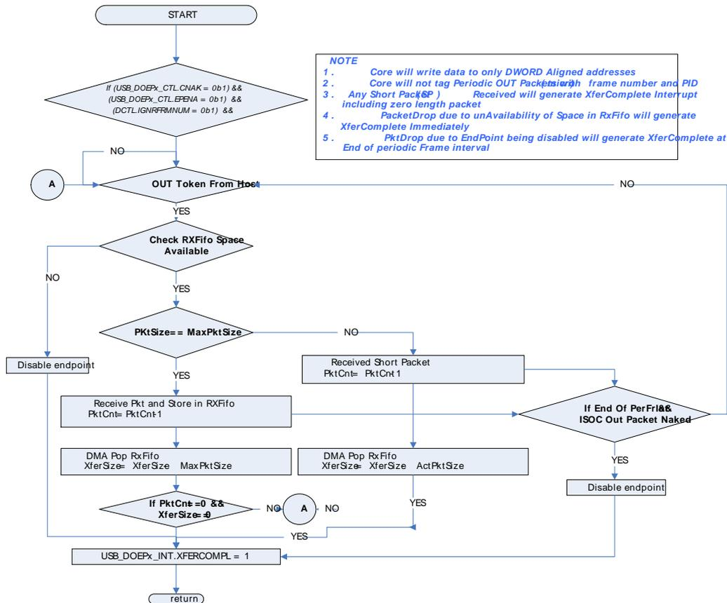
14.4.4.2.2.12 Incomplete Isochronous OUT Data Transfers in DMA and Slave Modes
