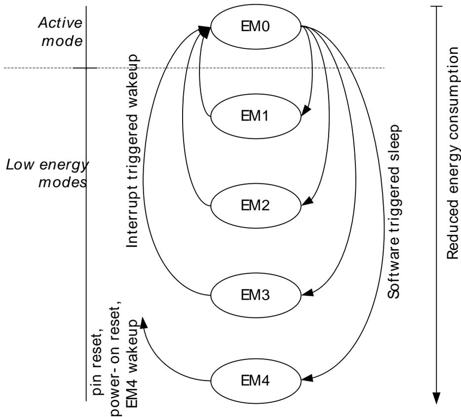
No direct transitions between EM1, EM2 or EM3 are available, as can also be seen from Figure 10.2 (p. 90) . Instead, a wakeup will transition back to EM0, in which software can enter any other low energy mode. An overview of the supported energy modes and the functionality available in each mode is shown in Table 10.1 (p. 91). Most peripheral functionality indicated as "On" in a particular energy mode can also be turned off from software in order to save further energy.
