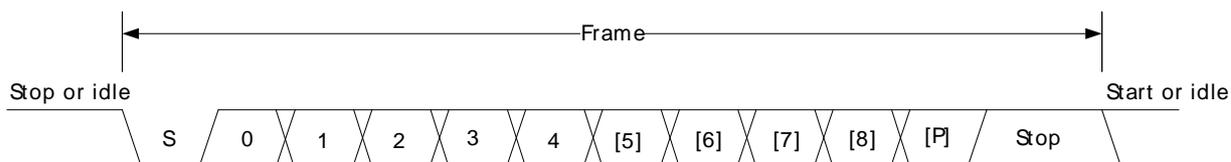
The number of data bits in a frame is set by DATABITS in USARTn\_FRAME, see Table 16.3 (p. 329) , and the number of stop-bits is set by STOPBITS in USARTn\_FRAME, see Table 16.4 (p. 329) . Whether or not a parity bit should be included, and whether it should be even or odd is defined by PARITY, also in USARTn\_FRAME. For communication to be possible, all parties of an asynchronous transfer must agree on the frame format being used.
