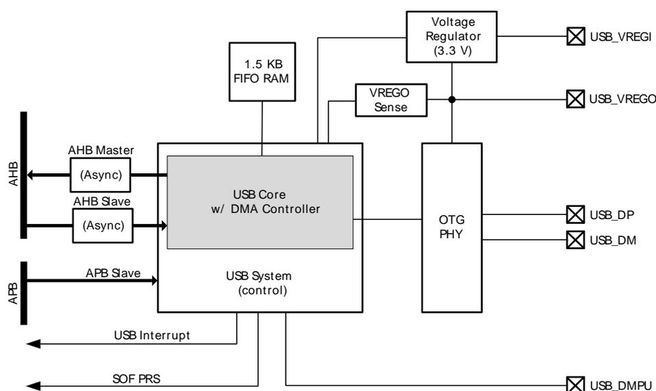
The USB consists of a digital logic part, an endpoint RAM, PHY and a voltage regulator with output voltage sensor. The voltage regulator provides a stable 3.3 V supply for the PHY, but can also be used to power the EFM32 itself as well as external components.
