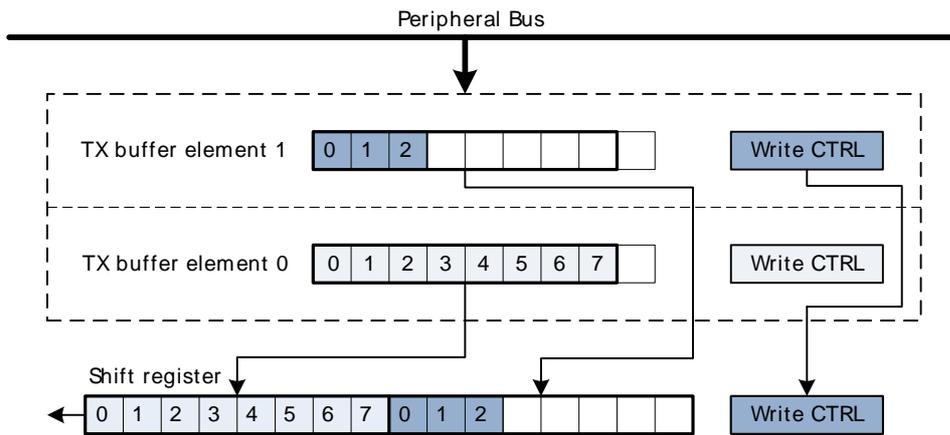
As shown in Figure 16.9 (p. 339), frame transmission control bits are taken from the second element in FIFO.
