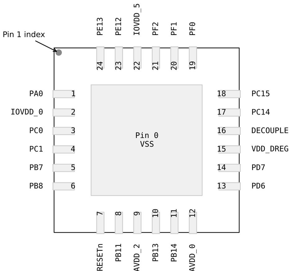
Figure 5.2. EFM32ZG110 Pinout (top view, not to scale)
