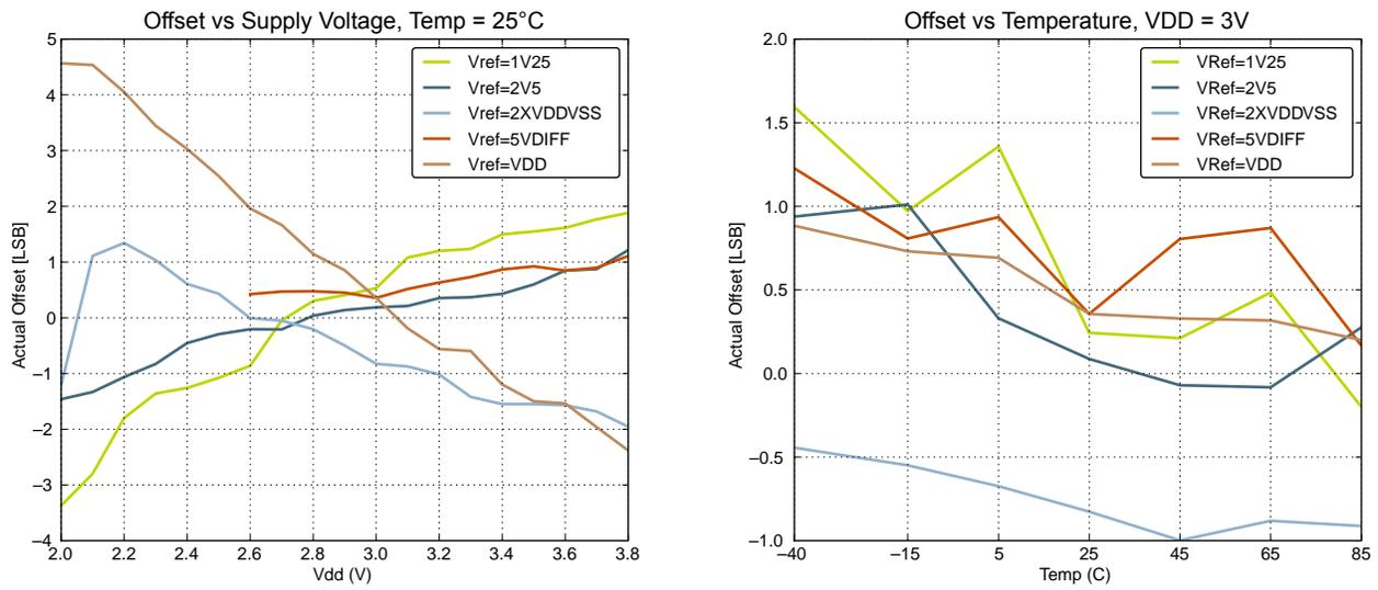
Figure 4.31. ADC Absolute Offset, Common Mode = VDD/2
