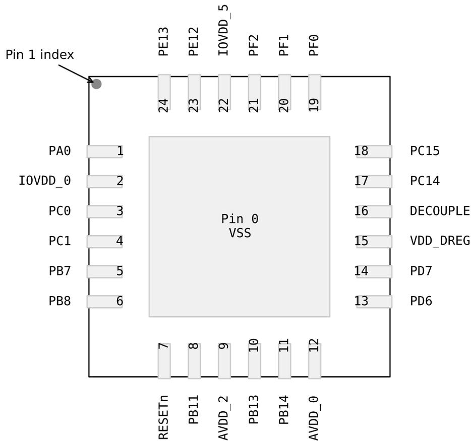
Figure 5.1. EFM32ZG108 Pinout (top view, not to scale)
