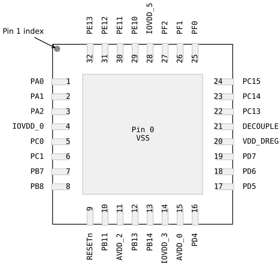
Figure 5.3. EFM32ZG210 Pinout (top view, not to scale)
