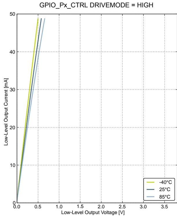
Figure 4.18. Typical Low-Level Output Current, 3.8 V Supply Voltage
