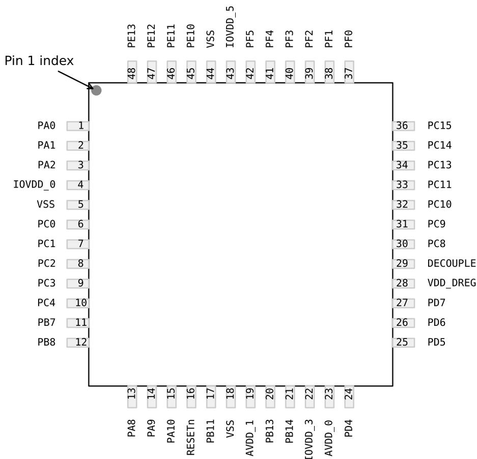
Figure 5.4. EFM32ZG222 Pinout (top view, not to scale)
