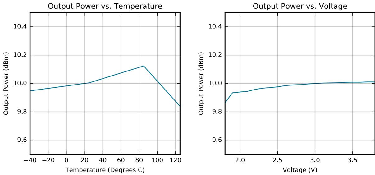
Figure 4.4. 2.4 GHz 10 dBm PA RF Transmitter Output Power
