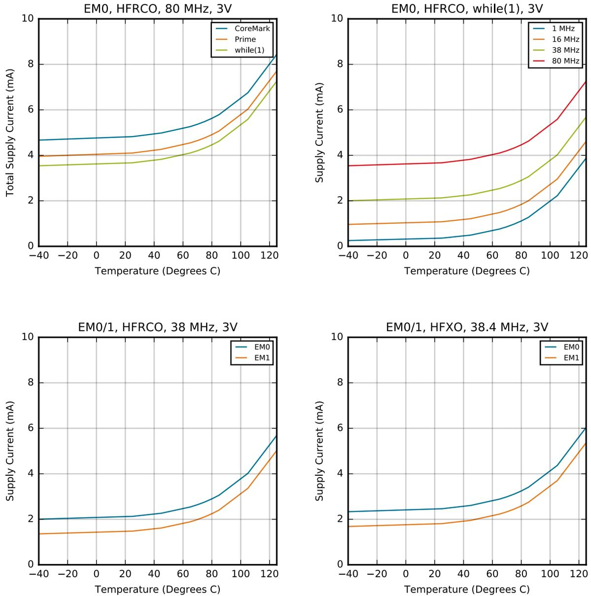
Figure 4.1. EM0 Active Mode Typical Supply Current vs. Temperature
