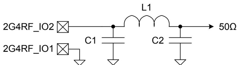
Figure 5.3. Typical 10 dBm 2.4 GHz RF impedance-matching network circuit
