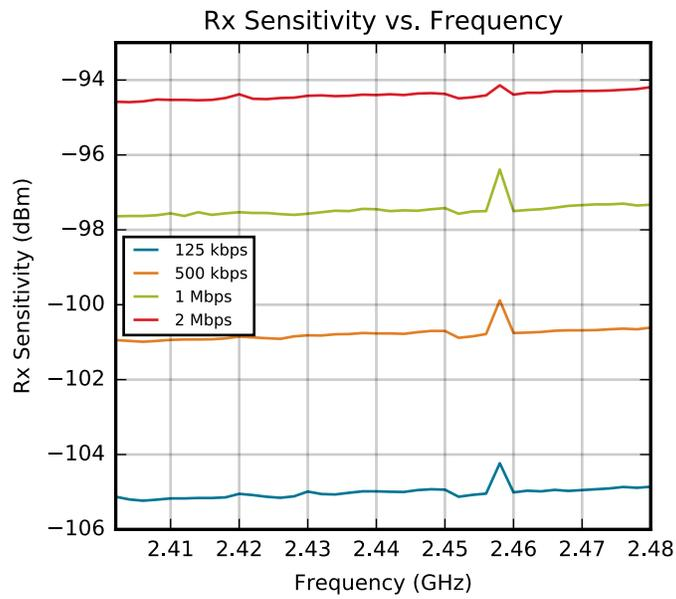
**Figure 4.6. 2.4 GHz BLE RF Receiver Sensitivity**
