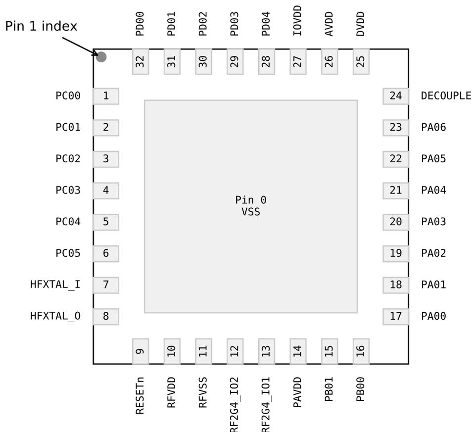
Figure 6.1. QFN32 2.4GHz Device Pinout
