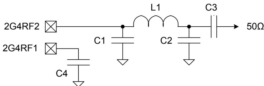
Figure 5.2. Typical 0 dBm 2.4 GHz RF impedance-matching network circuit
