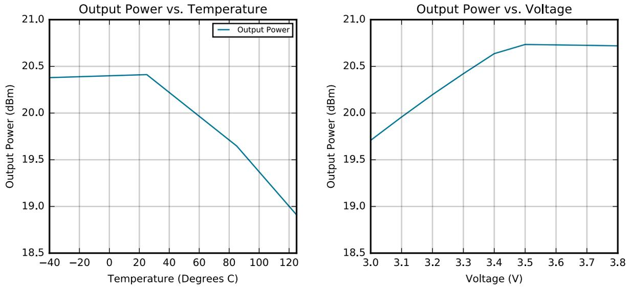
Figure 4.3. 2.4 GHz 20 dBm PA RF Transmitter Output Power
