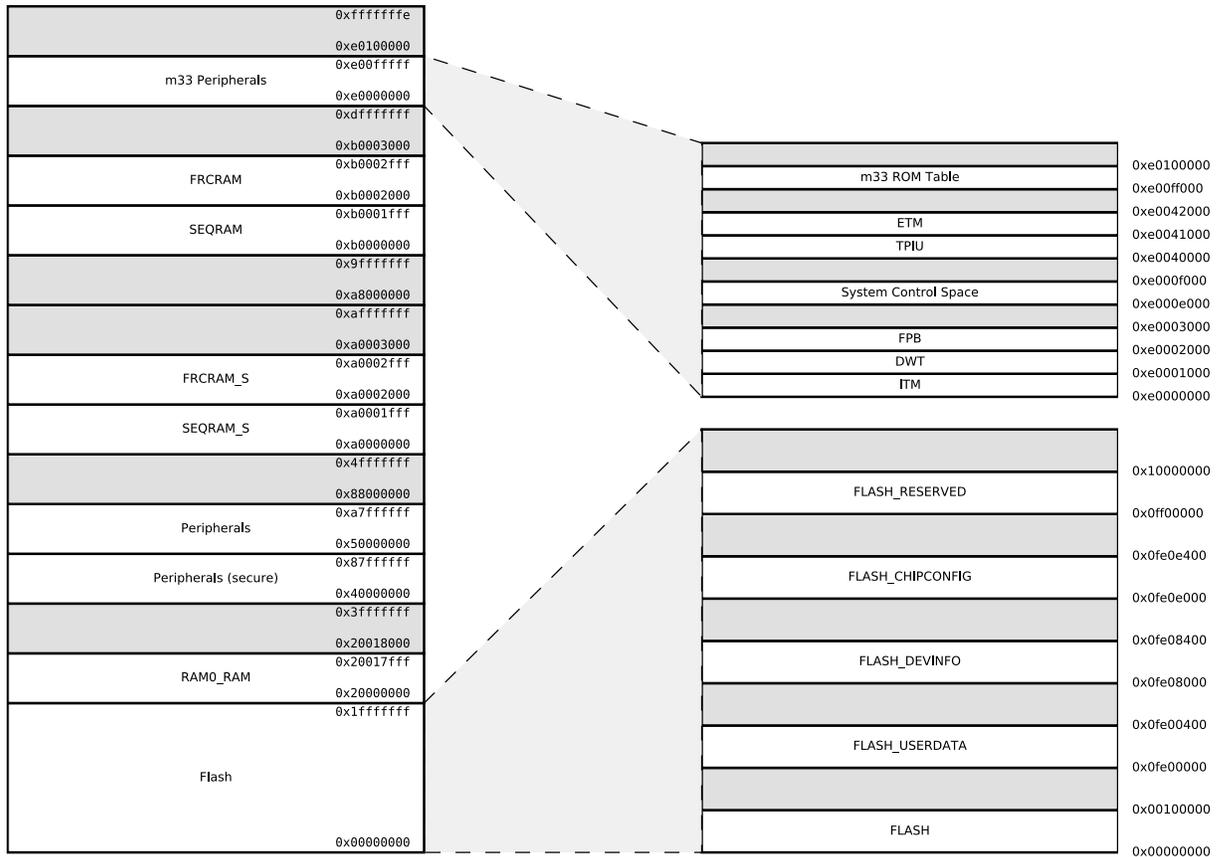
Figure 3.2. EFR32BG21 Memory Map — Core Peripherals and Code Space
