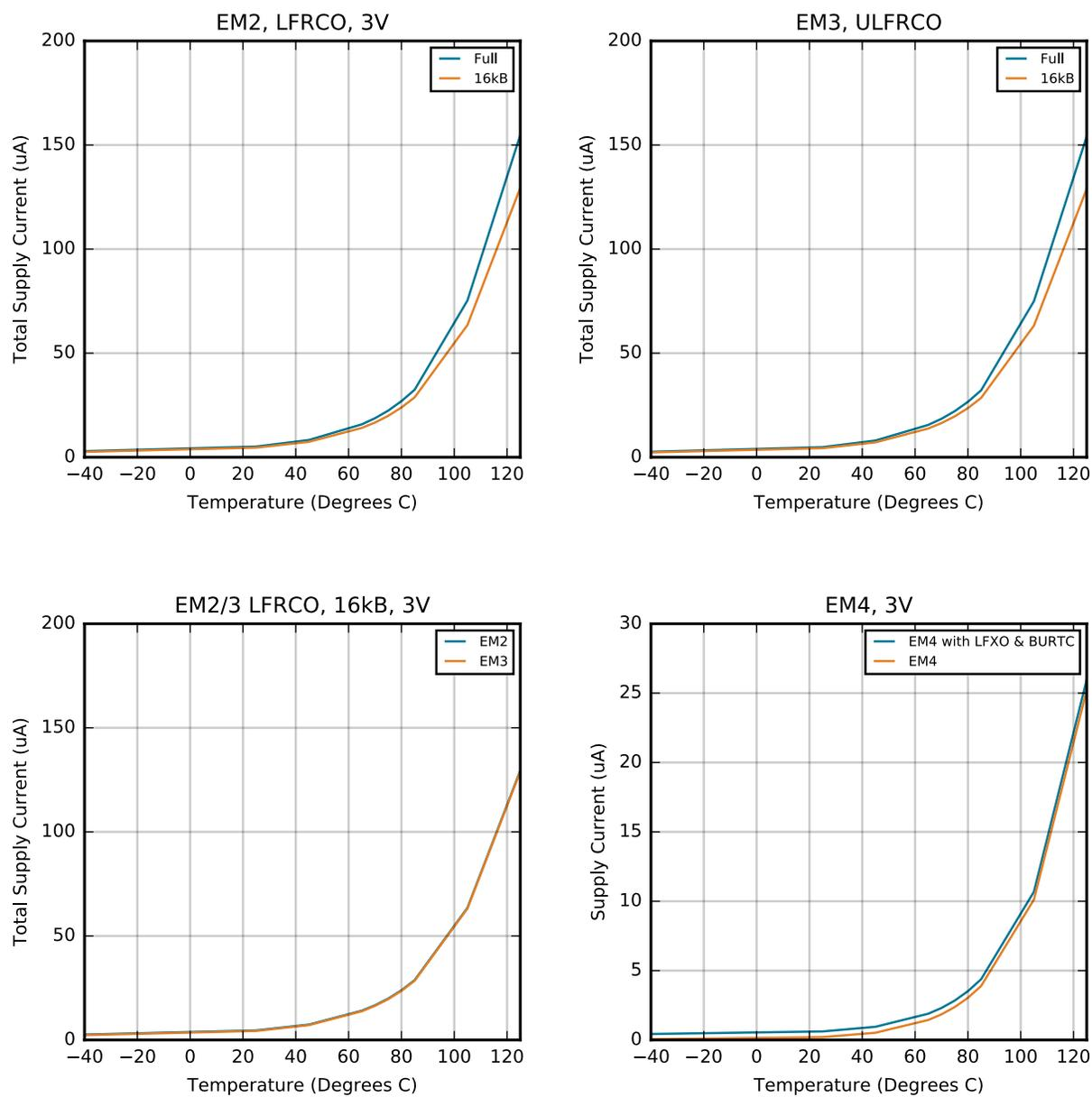
Figure 4.2. EM2, EM3, and EM4 Sleep Mode Typical Supply Current vs. Temperature
