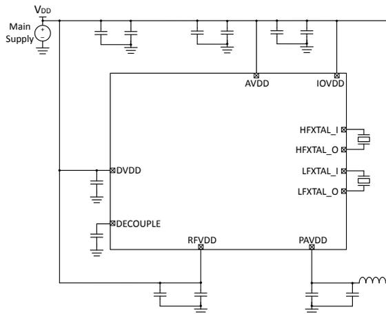
Figure 5.1. EFR32BG21 Typical Application Circuit: Direct Supply Configuration
