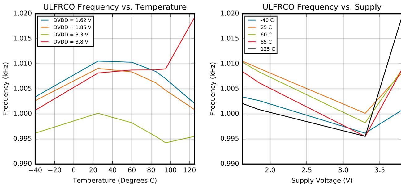
Figure 4.19. ULFRCO Typical Performance at 1 kHz
