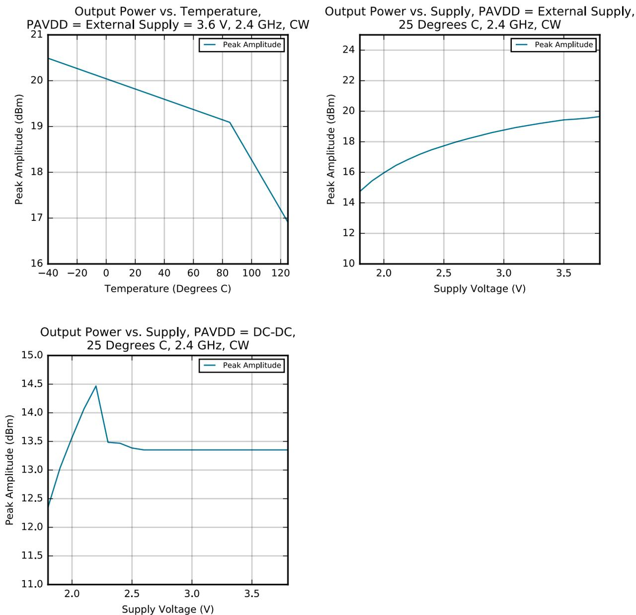
Figure 4.20. 2.4 GHz RF Transmitter Output Power
