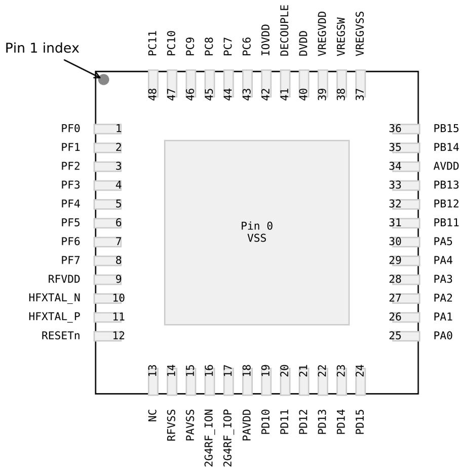
**Figure 6.2. QFN48 2.4 GHz Device Pinout**
