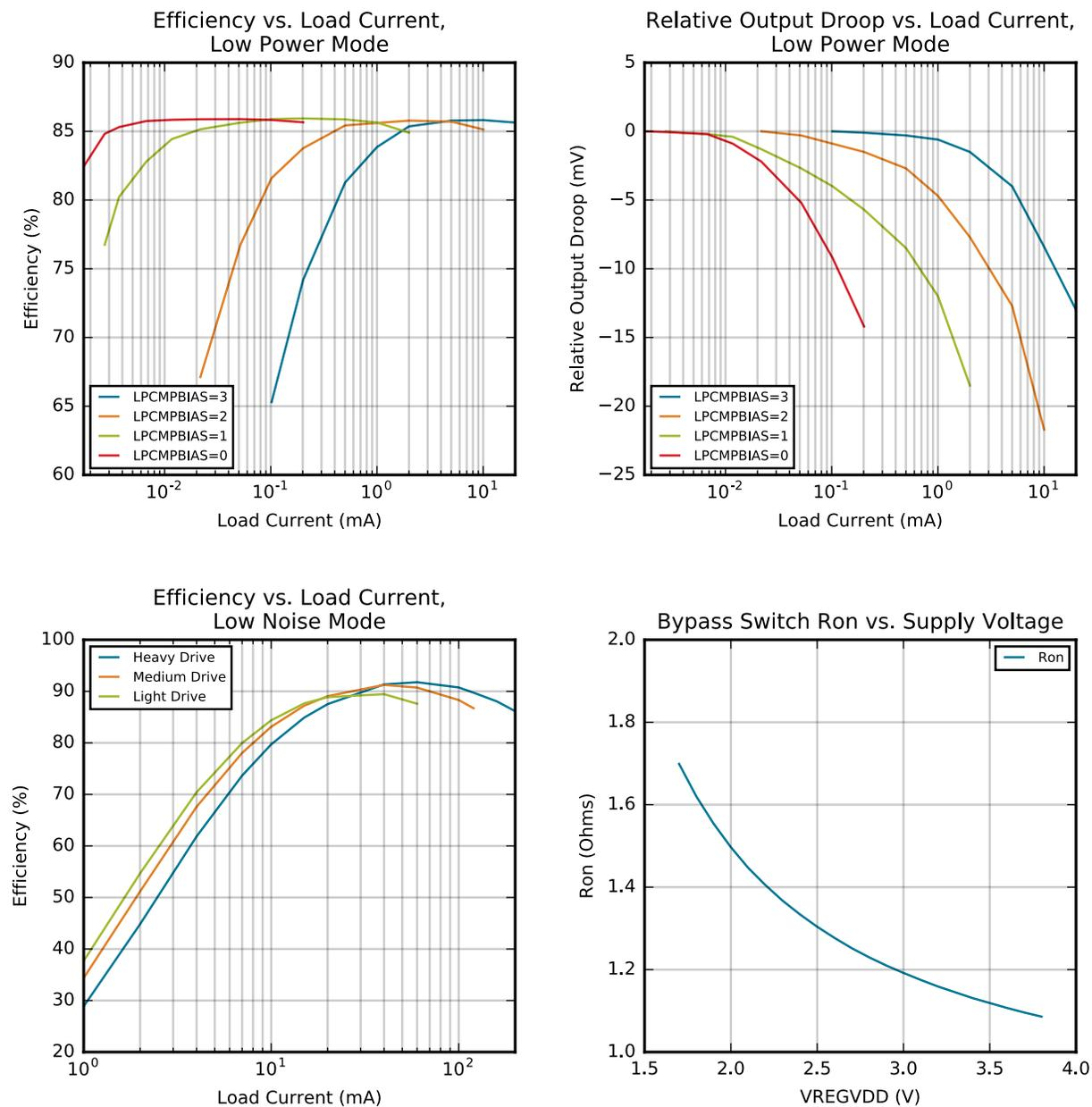
Figure 4.6. DC-DC Converter Typical Performance Characteristics
