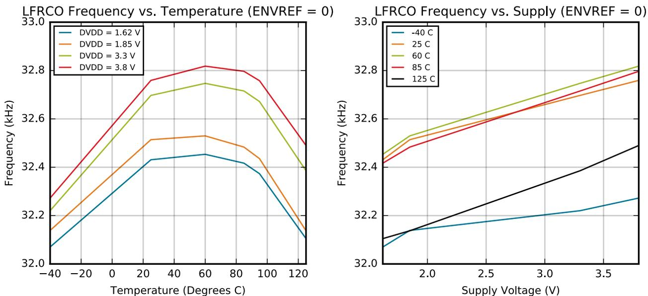
Figure 4.18. LFRCO Typical Performance at 32.768 kHz
