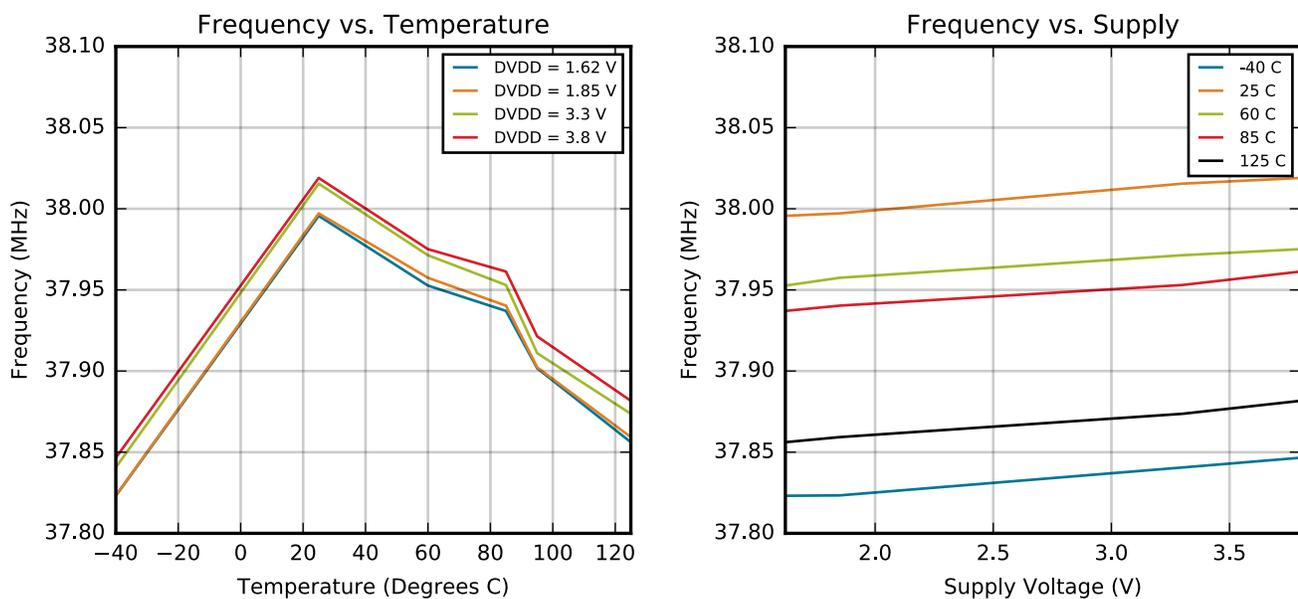
Figure 4.8. HFCO and AUXHFCO Typical Performance at 38 MHz
