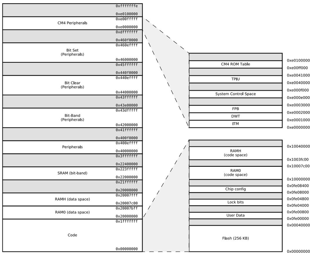
Figure 3.2. EFR32FG1 Memory Map — Core Peripherals and Code Space
