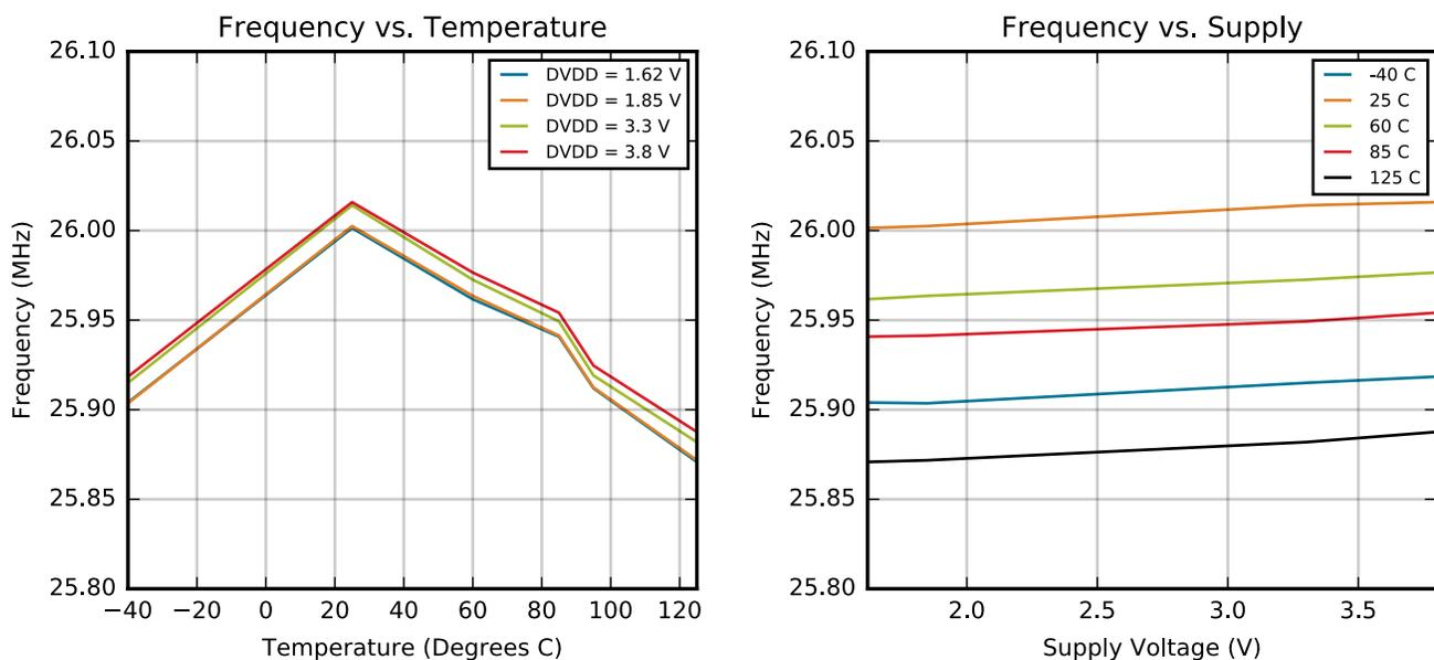
Figure 4.10. HFCO and AUXHFCO Typical Performance at 26 MHz
