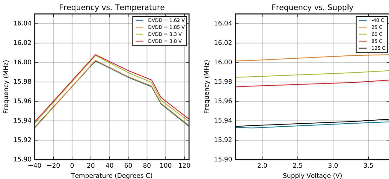
Figure 4.12. HFCO and AUXHFCO Typical Performance at 16 MHz
