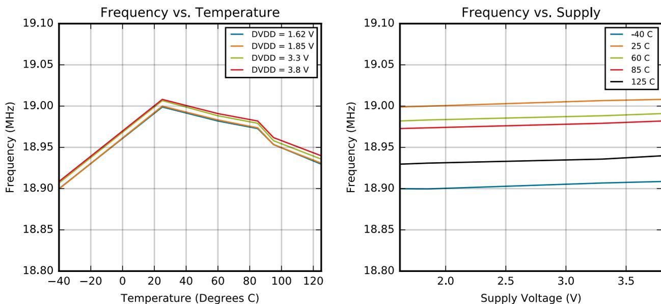
Figure 4.11. HFCO and AUXHFCO Typical Performance at 19 MHz
