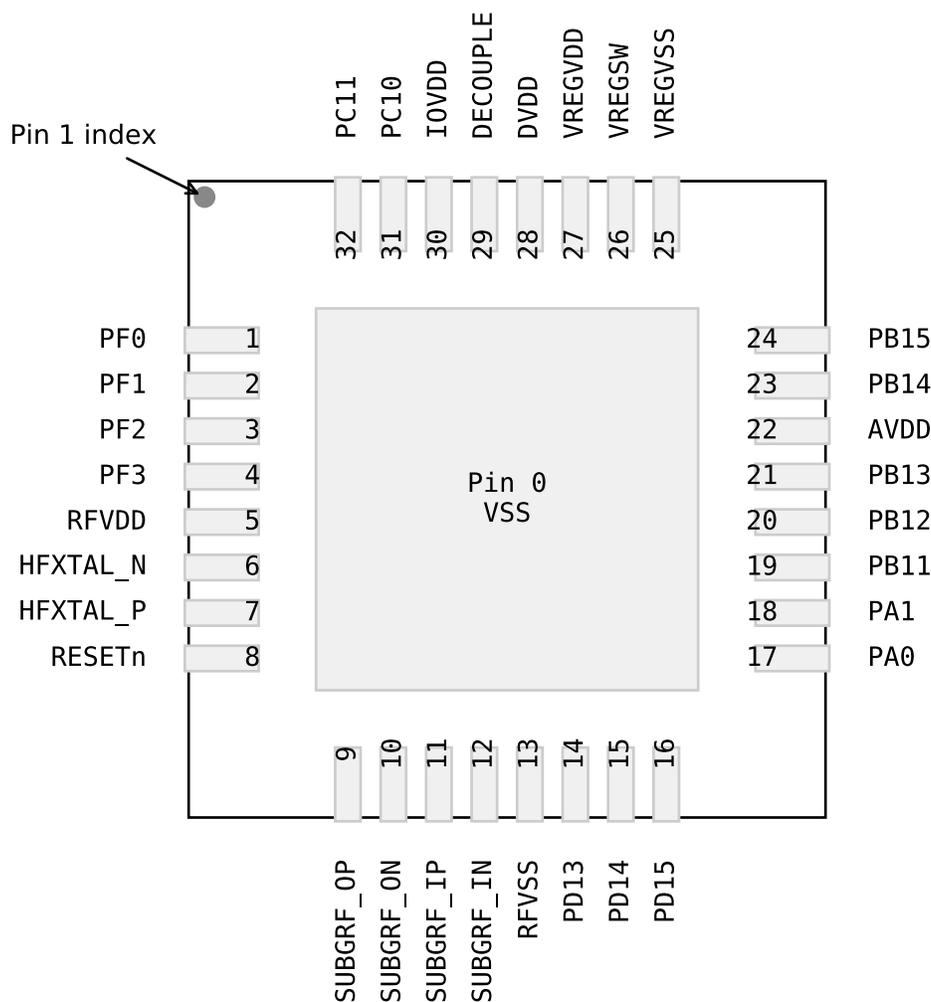
**Figure 6.5. QFN32 Sub-GHz Device Pinout**
