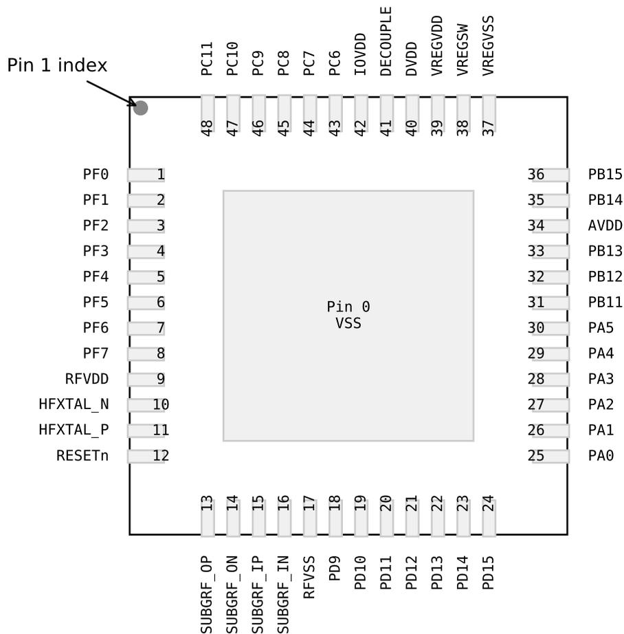
Figure 6.3. QFN48 Sub-GHz Device Pinout
