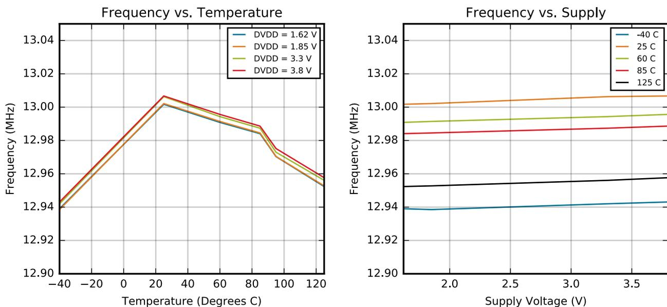
Figure 4.13. HFCO and AUXHFCO Typical Performance at 13 MHz
