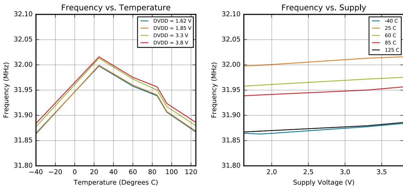
Figure 4.9. HFCO and AUXHFCO Typical Performance at 32 MHz
