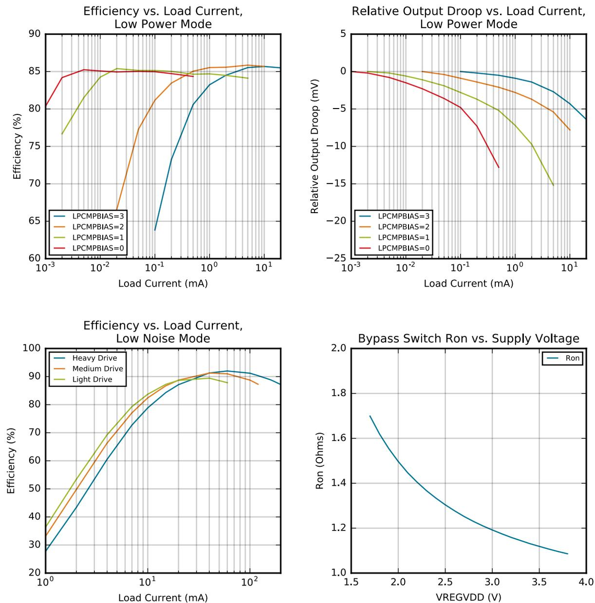
Figure 4.8. DC-DC Converter Typical Performance Characteristics
