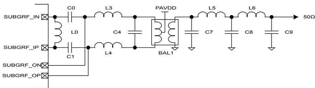
**Figure 5.5. Typical Sub-GHz RF impedance-matching network circuits**
