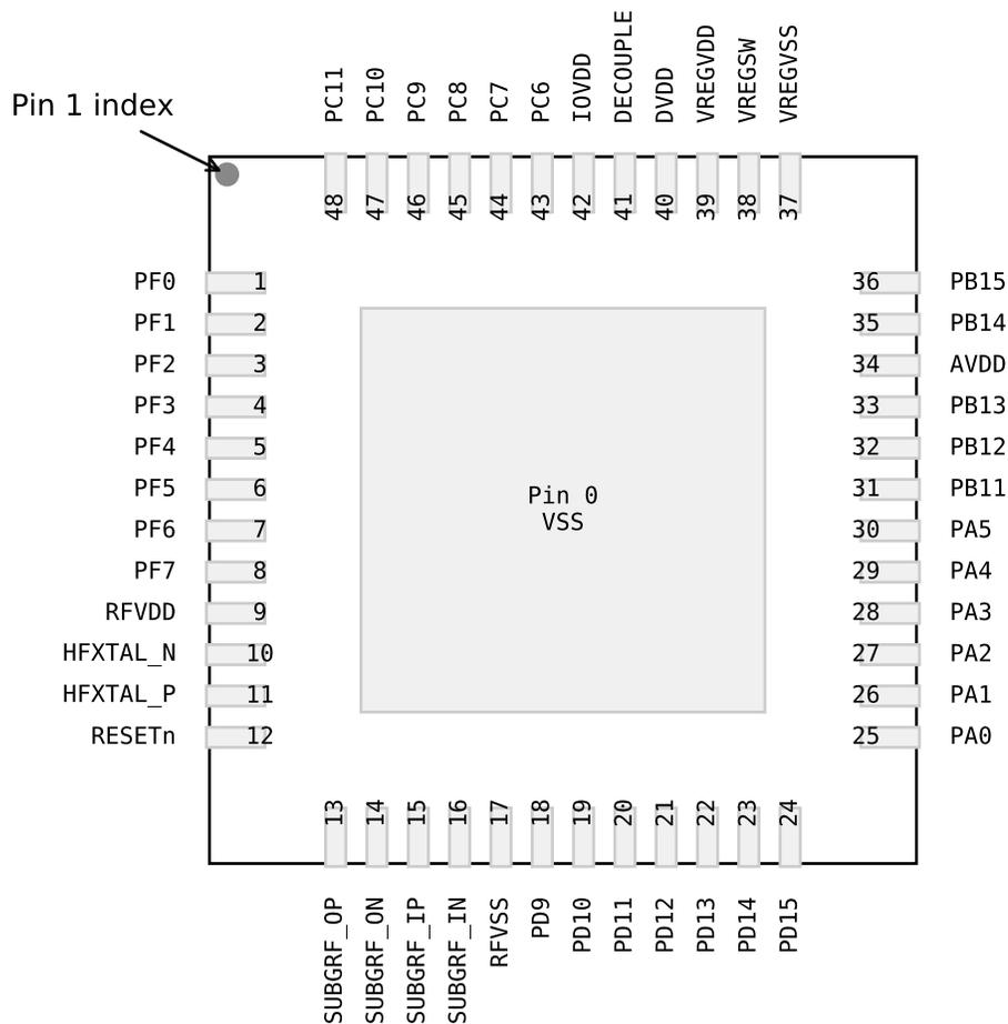
Figure 6.3. QFN48 Sub-GHz Device Pinout
