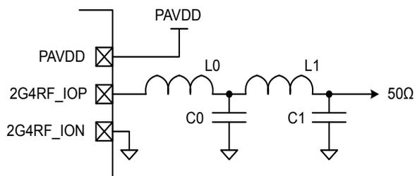
**Figure 5.4. Typical 2.4 GHz RF impedance-matching network circuits**
