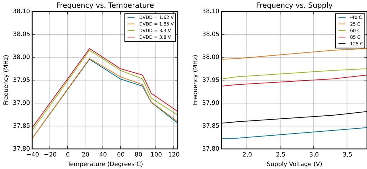
Figure 4.8. HFRCO and AUXHFRCO Typical Performance at 38 MHz
