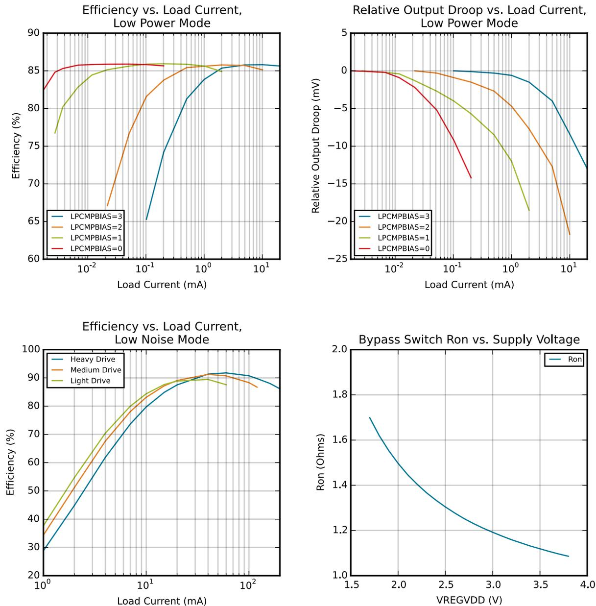
Figure 4.6. DC-DC Converter Typical Performance Characteristics
