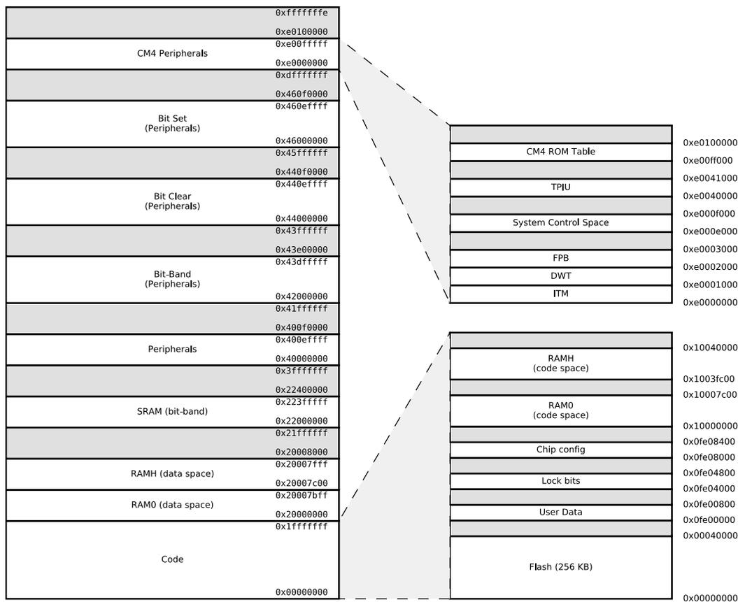
Figure 3.2. EFR32MG1 Memory Map — Core Peripherals and Code Space
