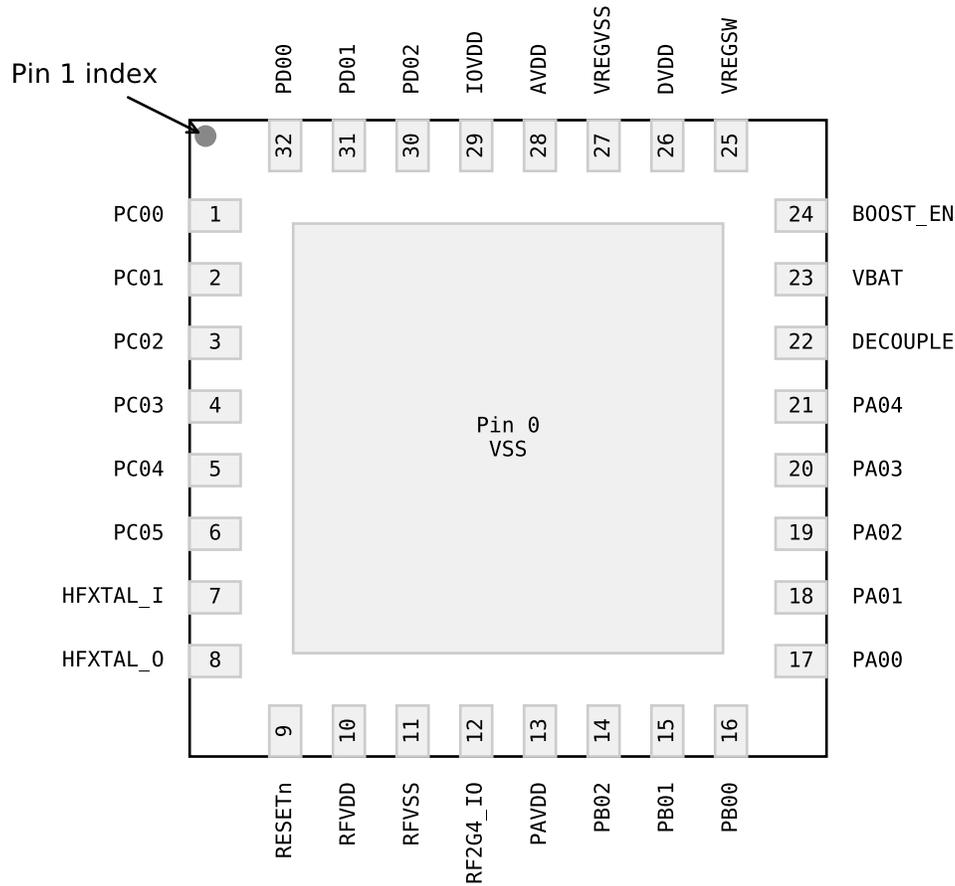
**Figure 6.4. QFN32 with Boost DC-DC Device Pinout**
