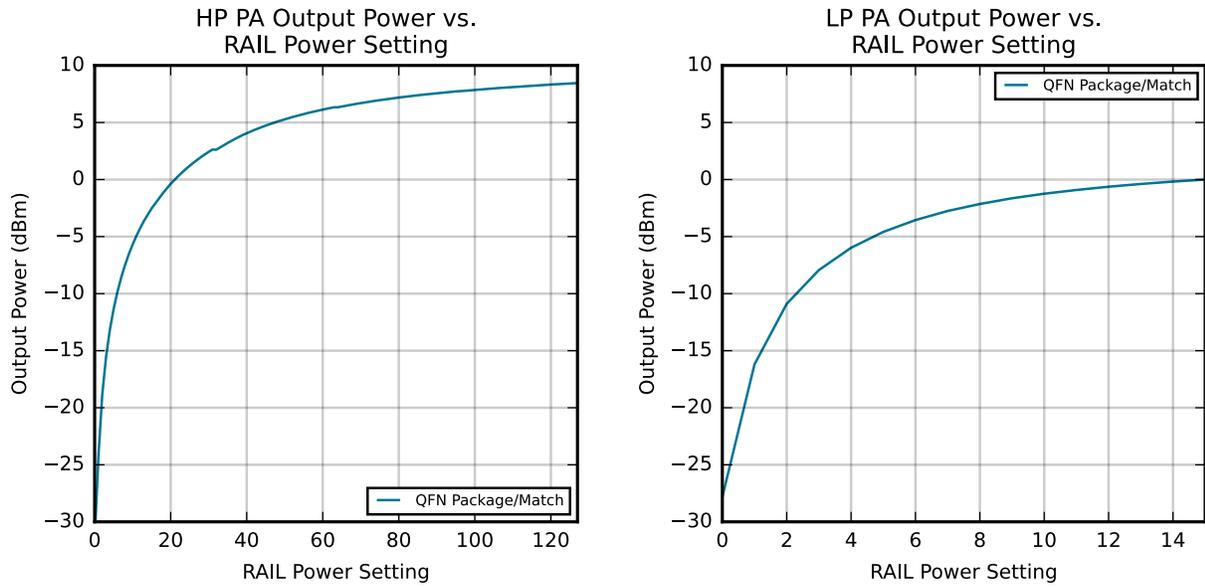
Figure 4.12. Transmitter Output Power, QFN Package / Matching
