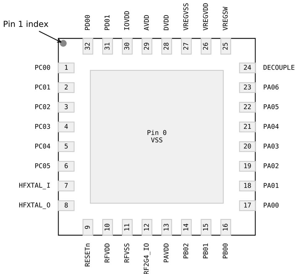
Figure 6.3. QFN32 with Buck DC-DC Device Pinout
