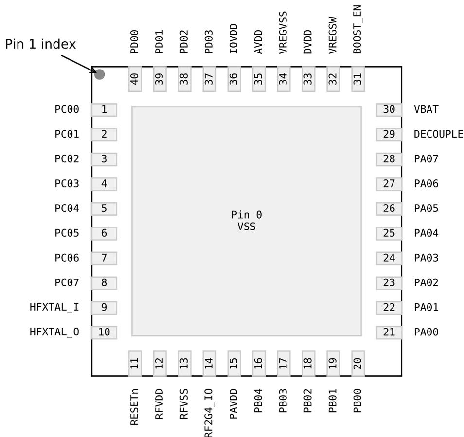
Figure 6.2. QFN40 with Boost DC-DC Device Pinout
