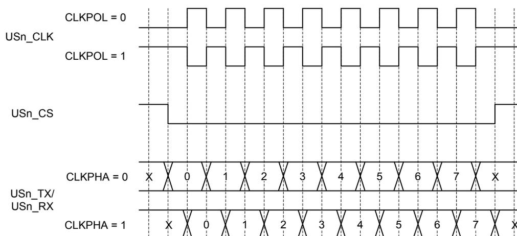
**Figure 18.20. USART SPI Timing**
