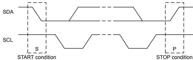
**Figure 17.4. I<sup>2</sup>C START and STOP Conditions**
