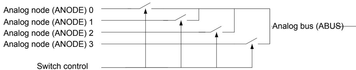
**Figure 33.1. Analog Bus (ABUS)**
