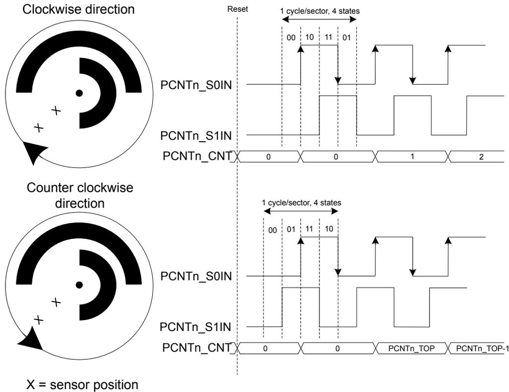
Figure 16.2. PCNT Quadrature Coding
