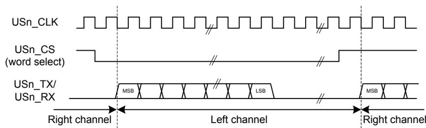
**Figure 18.22. USART Standard I2S Waveform (Reduced Accuracy)**
