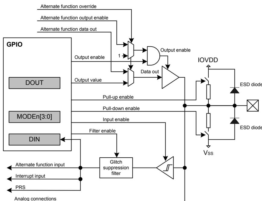
Figure 32.1. Pin Configuration
