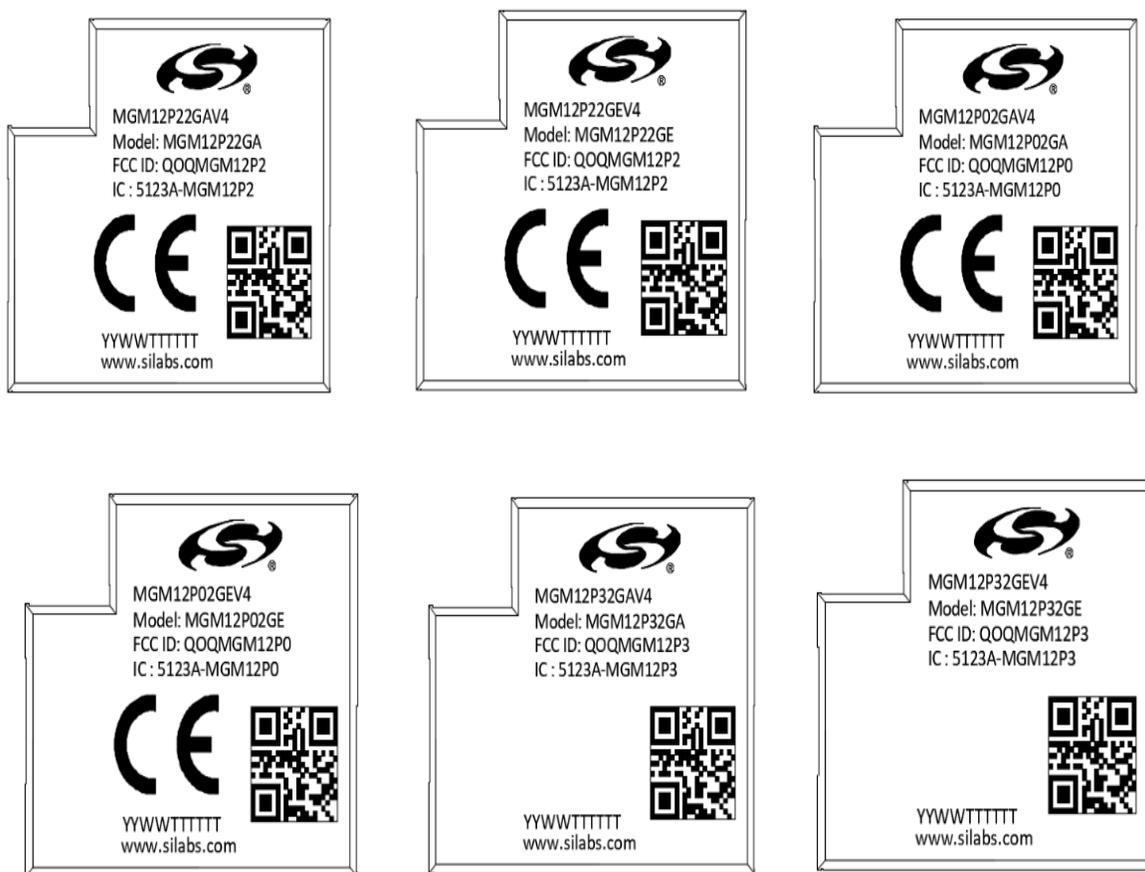
**Figure 9.5. MGM12P Package Marking**
