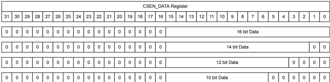
**Figure 34.6. Data Encoding for Different Resolution Settings**
