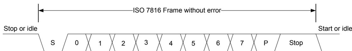
**Figure 18.15. USART ISO 7816 Data Frame Without Error**
