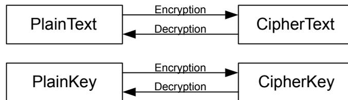
**Figure 31.4. CRYPTO Key and Data Definitions**
