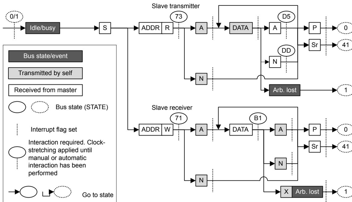
Figure 17.16. I<sup>2</sup>C Slave State Machine
