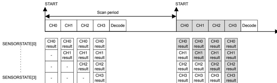
**Figure 28.10. Sensor Scan and Decode Sequence**
