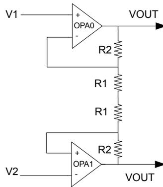
Figure 24.11. Instrumentation Amplifier Overview
