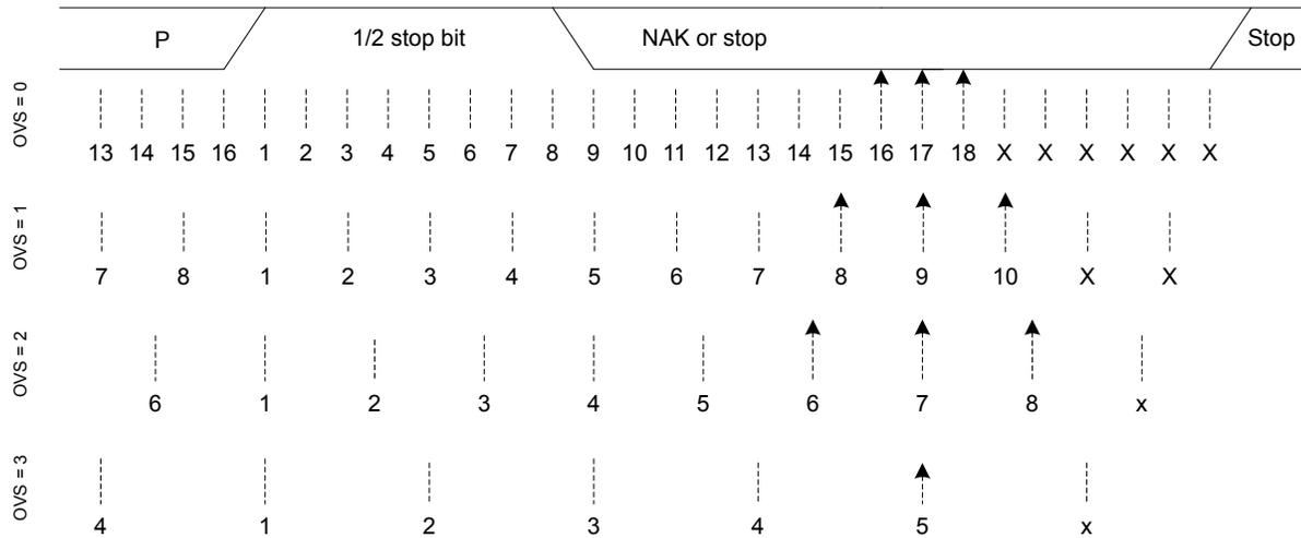
**Figure 18.17. USART SmartCard Stop Bit Sampling**
