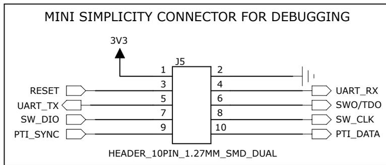
**Figure 5.1. MGM210L Application Schematic**
