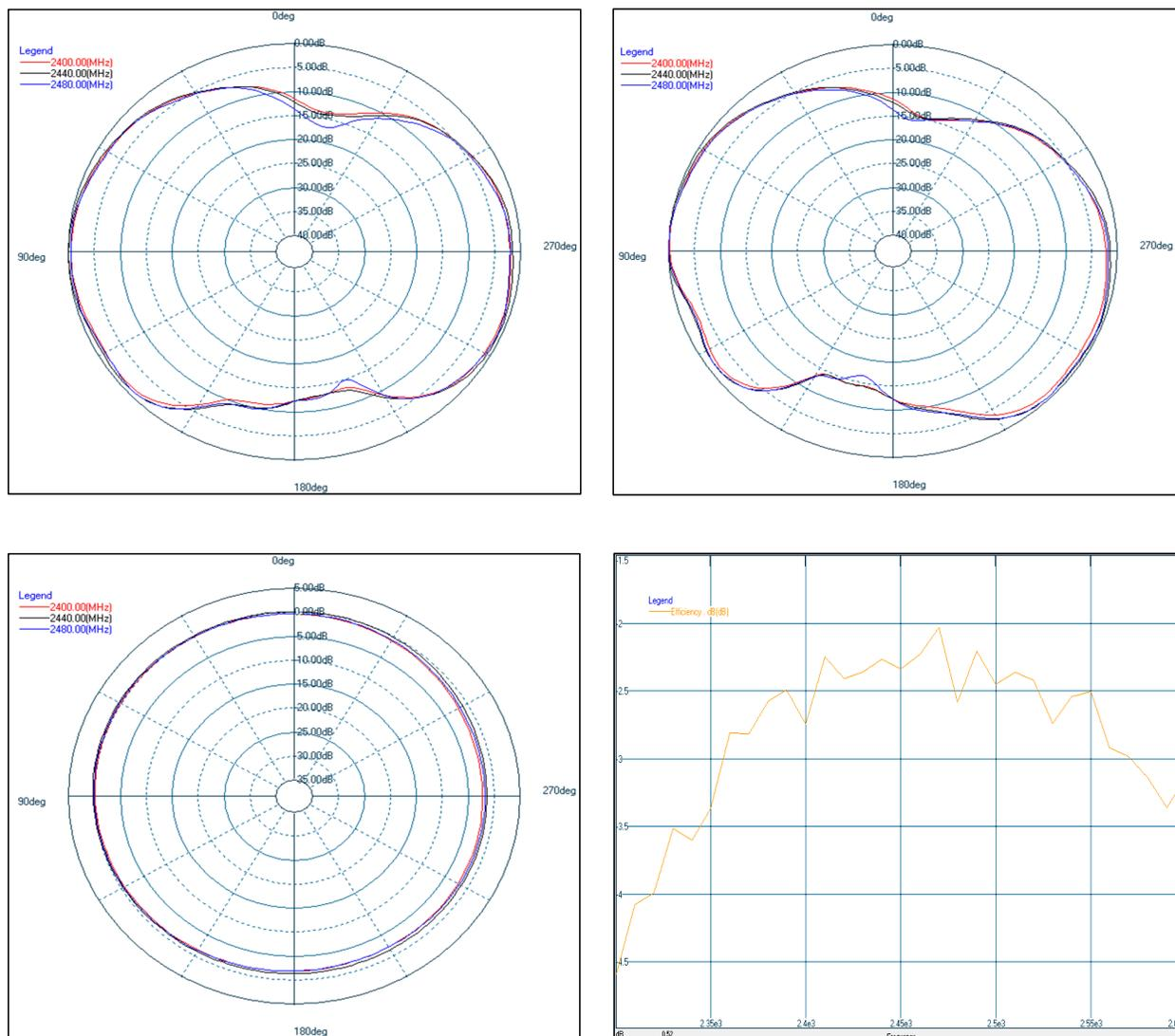
**Figure 4.1. Typical 2D Antenna Radiation Patterns and Efficiency**
