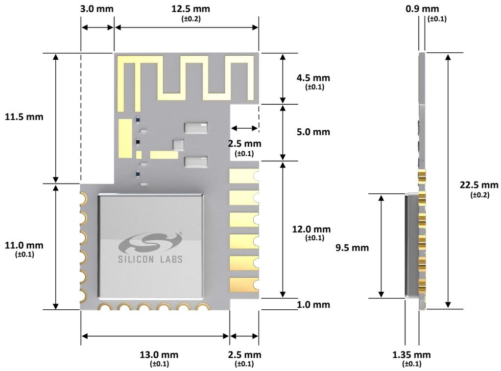
Figure 8.1. Module Dimensions
