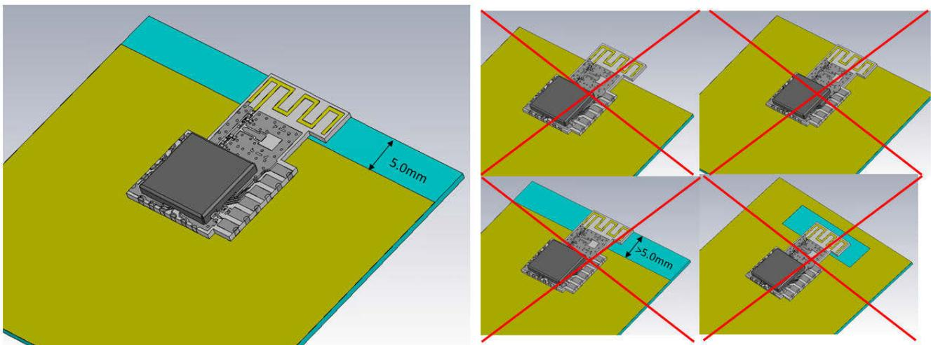
**Figure 7.2. Horizontal Mounting**
