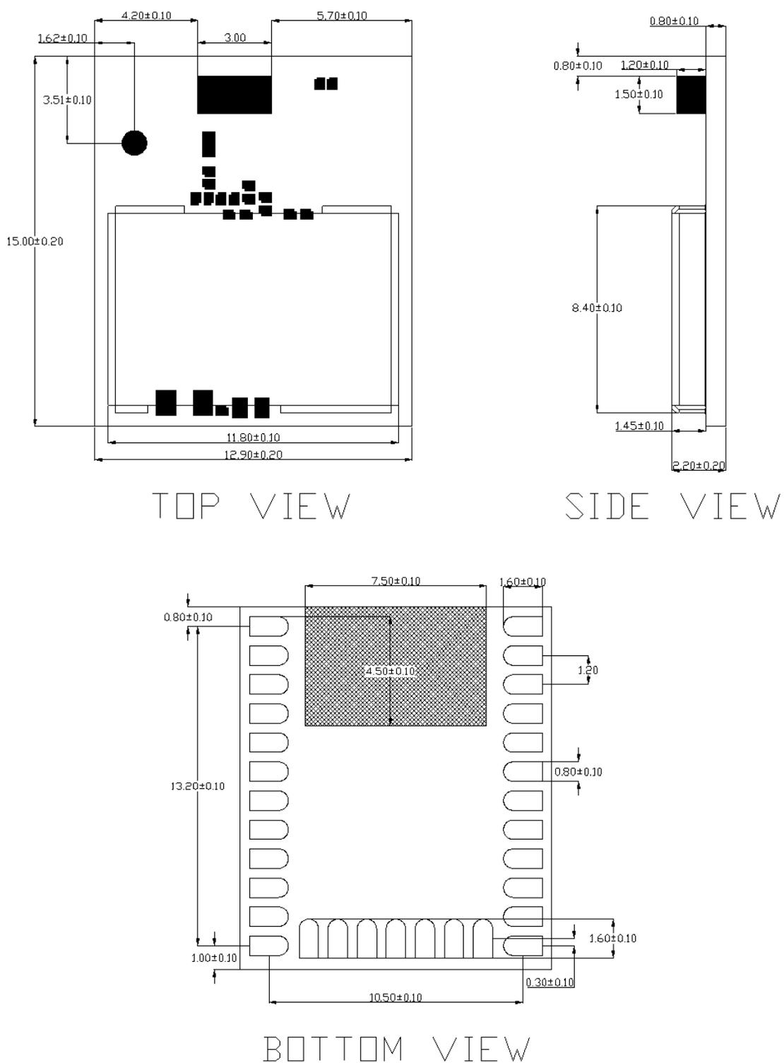
Figure 8.1. Module Dimensions
