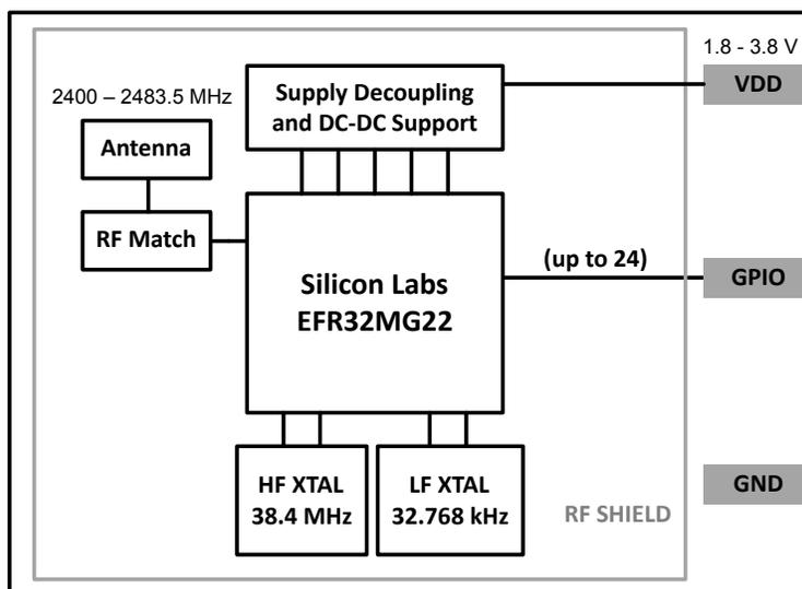
Figure 3.1. MGM220P Block Diagram
