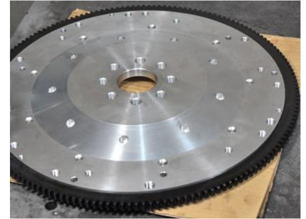
180 Teeth Ring Gear used for Timing
