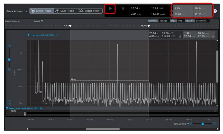
Figure 5-4 Energy profiler capture on a node operating in EM2 (deep sleep) mode for a given interval
