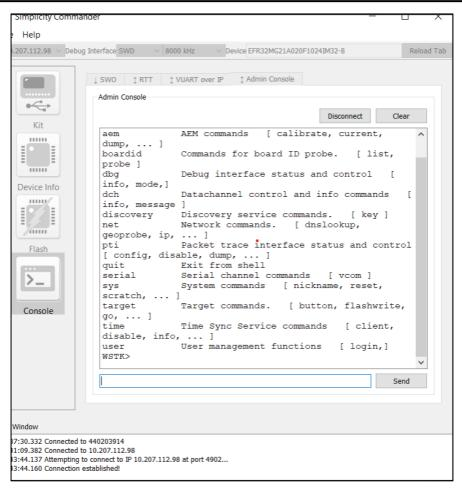
4. Next send the command "serial vcom config speed 921600"
