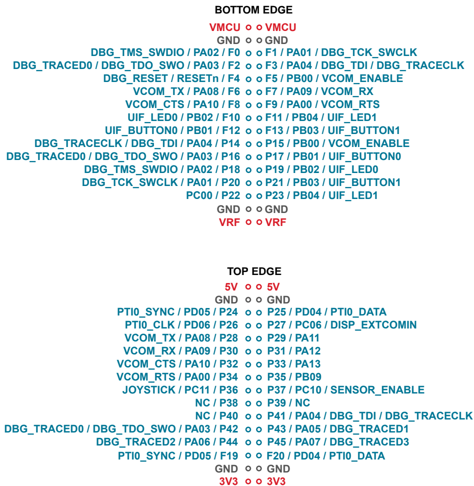
Figure 3.3. Wireless Pro Kit Mainboard (BRD4002A) Breakout Pad Pin Mapping
