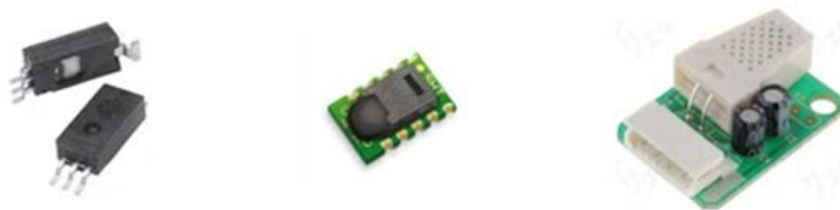
Figure 2. Examples of MCM/Hybrid/Module Humidity Sensor Solutions
