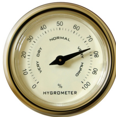
Figure 1. Hair Tension Dial Hygrometer with Nonlinear Scale
